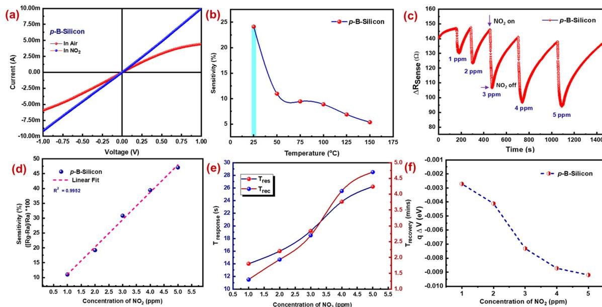
**Fig. 4** (a) Current–voltage characteristics of p-B-silicon, (b) response graph towards exposure to 2 ppm of NO<sub>2</sub> as a function of temperature for p-B-silicon, (c) dynamic NO<sub>2</sub> sensing characteristics of p-B-silicon, (d) NO<sub>2</sub> response as a function of concentration, (e) NO<sub>2</sub> response as a function of response and recovery time and (f) plot of variations in band bending energy of the p-B-silicon based sensor.
