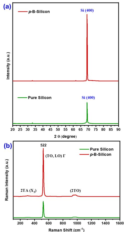
Fig. 3 (a) X-ray diffraction and (b) Raman spectra for pure silicon and the p-B-silicon device.
