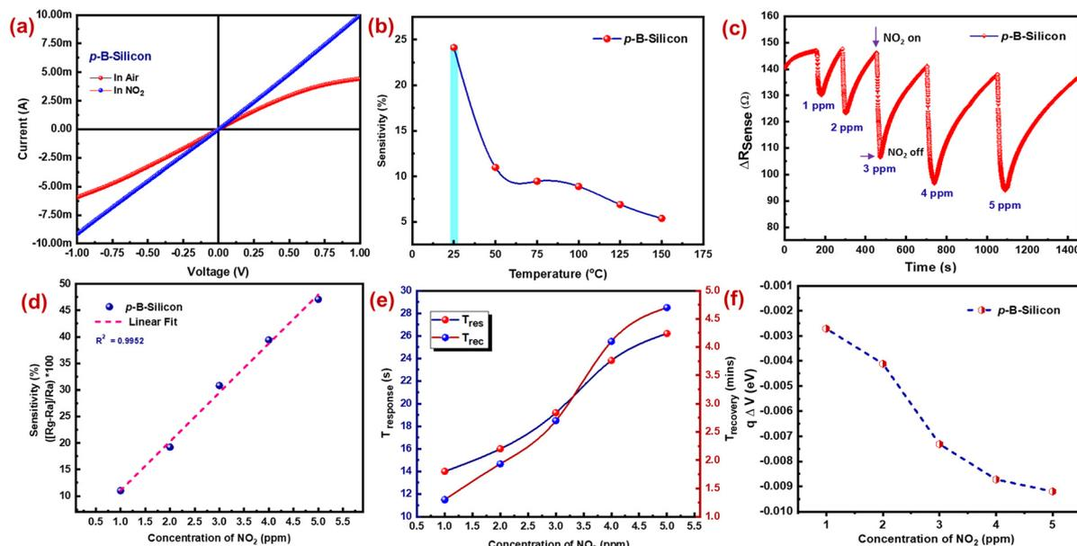
**Fig. 4** (a) Current–voltage characteristics of p-B-silicon, (b) response graph towards exposure to 2 ppm of NO<sub>2</sub> as a function of temperature for p-B-silicon, (c) dynamic NO<sub>2</sub> sensing characteristics of p-B-silicon, (d) NO<sub>2</sub> response as a function of concentration, (e) NO<sub>2</sub> response as a function of response and recovery time and (f) plot of variations in band bending energy of the p-B-silicon based sensor.
