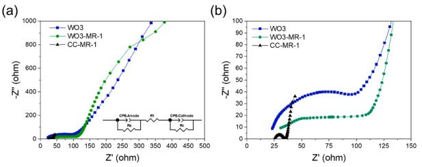
Fig. 4 (a) Electrochemical impedance plots of electrodes of CC-MR-1, WO<sub>3</sub> and WO<sub>3</sub>-MR-1 with an equivalent circuit model used to fit experimental data; (b) enlarged electrochemical impedance plots of (a).
