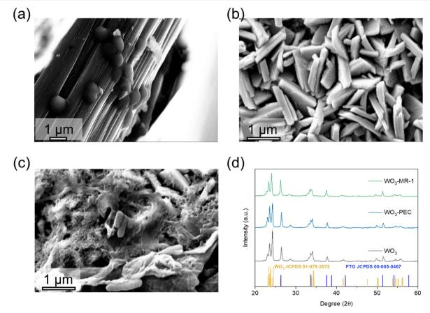
Fig. 1 SEM image of (a) carbon cloth (CC) with MR-1, (b) WO<sub>3</sub> and (c) WO<sub>3</sub> with MR-1. The white rectangular bar on the bottom left-hand corner of each graph indicates the dimensions with 1 μm. (d) XRD patterns of WO<sub>3</sub>, WO<sub>3</sub> photoelectrode, and WO<sub>3</sub>-MR-1 biophotoelectrode.
