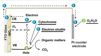
Fig. 5 Schematic diagram of the photocurrent generation by the WO<sub>3</sub> electrode with MR-1 bacteria. FL, CB, and VB represent the fermi level, conduction, and valence bands, respectively.
