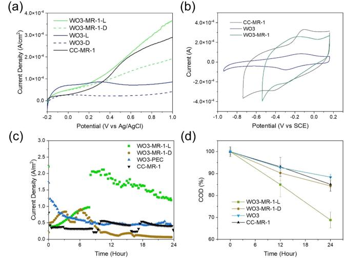
Fig. 2 (a) LSV, (b) CV, and (c) i-t curve under external bias of 0.8 V of S-MPEC using CC-MR-1, WO<sub>3</sub>, and WO<sub>3</sub>-MR-1 as anode under dark and light conditions. (d) Record of COD in the percentage of S-MPEC using CC-MR-1, WO<sub>3</sub>, and WO<sub>3</sub>-MR-1 as an anode.
