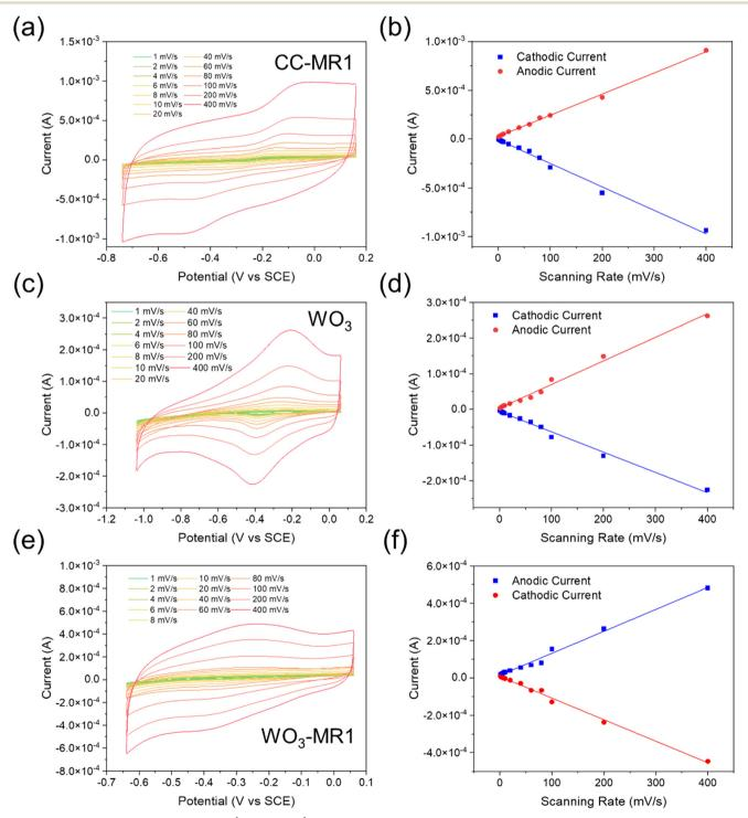
Fig. 3 CV at different scan rates from 1 mV  $s^{-1}$  to 40 mV  $s^{-1}$  of (a) CC-MR-1, (c) WO<sub>3</sub>, and (e) WO<sub>3</sub>-MR-1; peak current vs. scan rate plot of (b) CC-MR-1, (c) WO<sub>3</sub>-MR-1 is peak current vs. MR-1, (d)  $WO_3$  and (f)  $WO_3$ -MR-1.
