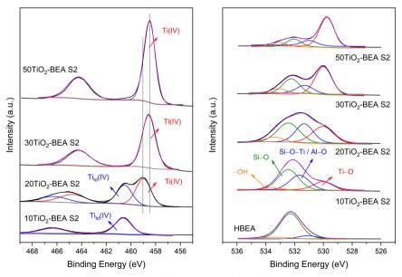
Fig. 9 XPS spectra of S2 series samples. Left: Ti2p core-level region; right side: O1s region.
