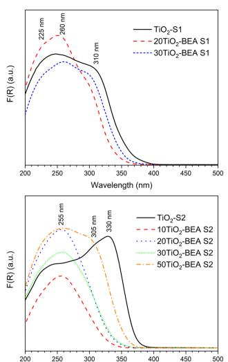
Fig. 7 UV-vis DRS spectra of series S1 (top) and S2 (bottom) composite materials
