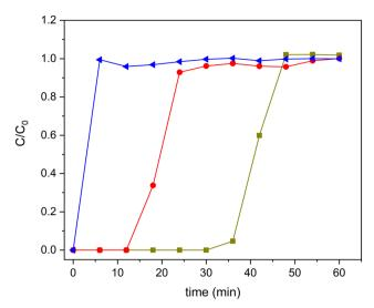
Fig. 10 Ethylene adsorption curves for samples H-BEA ( ), 20TiO<sub>2</sub>-BEA S2 ( $\bullet$ ) and TiO<sub>2</sub>-S2 ( $\blacktriangleleft$ ) (C<sub>2</sub>H<sub>4</sub> 100 ppm, 25 cm<sup>3</sup> min<sup>-1</sup>, RT)
