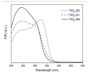
Fig. 2 UV-vis DRS spectra of bulk TiO<sub>2</sub> samples: TiO<sub>2</sub>-SA (black), TiO<sub>2</sub>-S1 (blue) and TiO2-S2 (red).
