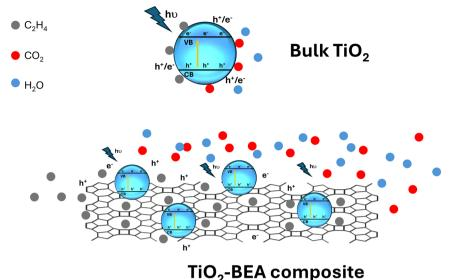
Scheme 1 Illustration of the adsorption and the photocatalytic degradation of ethylene on the surface of bulk TiO2 vs. zeolite-based TiO2 composites.
