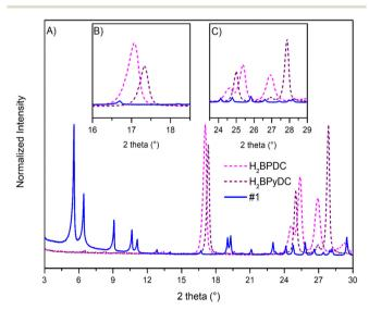
Fig. 1 A) PXRD pattern of #1 Ce-UiO-67-5% BPyDC (blue line) compared to those of the linkers H2BPDC (dashed pink line) and H<sub>2</sub>ByPDC (dashed violet line), showing no unreacted linkers residues. B) and C) show magnifications of the same PXRD patterns. For the MOF, intensities normalized to the 5.58° peak.
