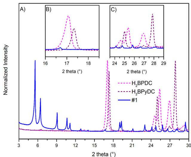
**Fig. 1** A) PXRD pattern of #1 Ce-UiO-67-5% BPyDC (blue line) compared to those of the linkers H<sub>2</sub>BPDC (dashed pink line) and H<sub>2</sub>BPyDC (dashed violet line), showing no unreacted linker residues. B) and C) show magnifications of the same PXRD patterns. For the MOF, intensities normalized to the 5.58° peak.
