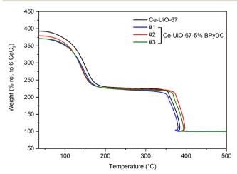
Fig. 3 TGA profiles of the three batches of Ce-UiO-67-5% BPyDC, #1 (blue line), #2 (red line) and #3 (green line), compared to that of Ce-UiO-67 (black line), reported as weight loss (%) related to CeO<sub>2</sub>, set as
