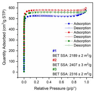
Fig. 4 N<sub>2</sub> adsorption-desorption isotherms at 77 K for the three batches of Ce-UiO-67-5% BPyDC: #1 in blue, #2 in red and #3 in green, respectively. For the sake of clarity, we have selected one of each three adsorption points up to 150 cm<sup>3</sup> g<sup>-1</sup> STP and then one every other.
