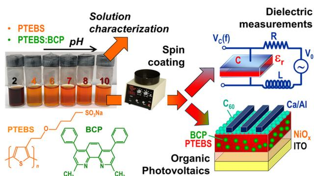
**Fig. 1** Flow-chart of the experiments described in this work, in which the pH of PTEBS solutions was varied from 2 to 10, with reproducible change in solution color at pH = 2, and subsequent solution characterization, fabrication of thin solid films by spin-coating and their characterization with a focus on dielectric function measurements, as well as organic photovoltaic device fabrication and testing.
