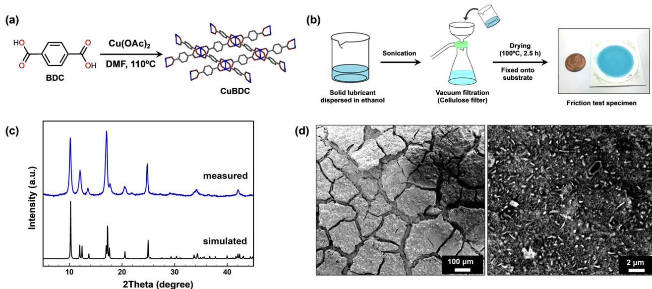
**Fig. 2** Preparation of the CuBDC-supported specimen: (a) synthesis of CuBDC using a solvothermal method; (b) preparation procedure of the specimens supporting the powder; (c) measured and simulated powder X-ray diffraction patterns of CuBDC, in which the latter one was calculated based on the single-crystal structure reported in ref. 25; (d) scanning electron microscopy (SEM) images of the surface of the CuBDC-supported specimen.
