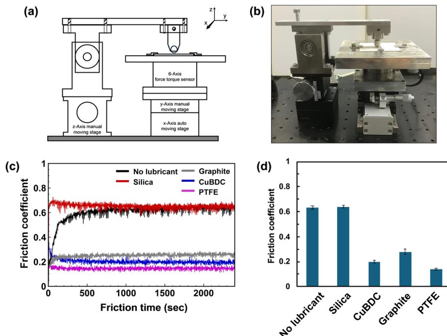
**Fig. 3** Characterization of the solid tribological properties on the powder-supported specimens: (a and b) schematic and optical images of the reciprocating tribometer; (c) friction coefficient vs. time curves of the specimens against a steel-ball counterpart; (d) friction coefficient of the specimens at the steady state (error bar: standard deviation).
