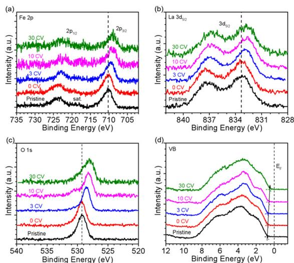
**Fig. 3** SXPS of LaFeO<sub>3</sub> with kinetic energy constant at 550 eV. (a) Fe 2p, (b) La 3d, (c) O 1s and (d) VB spectra after different CV cycles.
