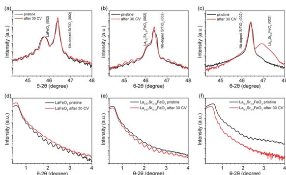
**Fig. 1** XRD and XRR of La<sub>1-x</sub>Sr<sub>x</sub>FeO<sub>3</sub> thin films in pristine state (black curves) and after 30 CV cycles (red curves). (a) XRD of LaFeO<sub>3</sub>, (b) XRD of La<sub>0.67</sub>Sr<sub>0.33</sub>FeO<sub>3</sub>, (c) XRD of La<sub>0.2</sub>Sr<sub>0.8</sub>FeO<sub>3</sub>, (d) XRR of LaFeO<sub>3</sub>, (e) XRR of La<sub>0.67</sub>Sr<sub>0.33</sub>FeO<sub>3</sub> and (f) XRR of La<sub>0.2</sub>Sr<sub>0.8</sub>FeO<sub>3</sub>.
