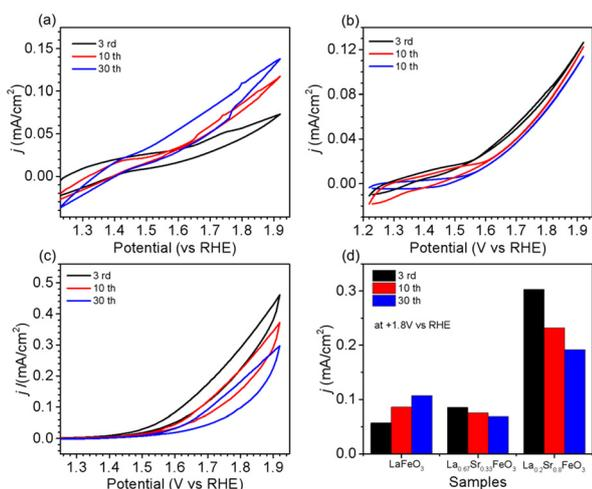
Fig. 5 OER performance of  $\text{La}_{1-x}\text{Sr}_x\text{FeO}_3$  with different CV cycles. (a) CV polarization curves of  $\text{LaFeO}_3$ , (b) CV polarization curves of  $\text{La}_{0.67}\text{Sr}_{0.33}\text{FeO}_3$ , (c) CV polarization curves of  $\text{La}_{0.2}\text{Sr}_{0.8}\text{FeO}_3$  and (d) current density of  $\text{La}_{1-x}\text{Sr}_x\text{FeO}_3$  ( $x = 0, 0.33, 0.8$ ) with different CV cycles at +1.8 V (vs. RHE).
