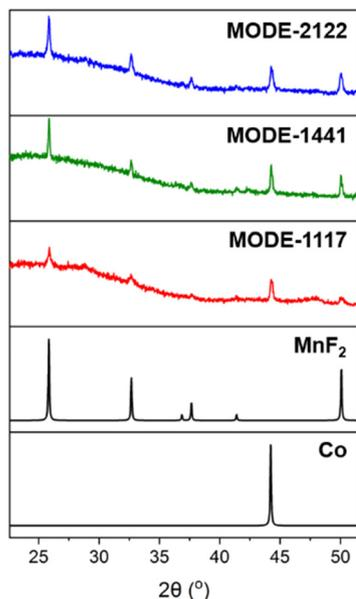
**Fig. 1** Comparison of the experimental PXRD patterns for MODEs-2122 (blue), -1441 (green), and -1117 (red) with the calculated PXRD patterns (black) for  $\text{MnF}_2$  (PDF 01-083-2417) and Co (PDF 00-015-0806).
