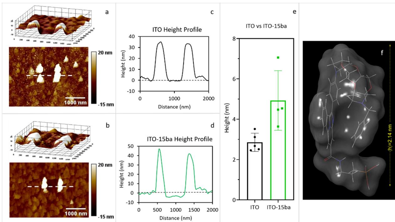
**Fig. 4** a) Representative 3D and 2D topography images of a scratched ITO surface area. b) Representative 3D and 2D topography images of a scratched ITO-15ba surface area. c) Cross section of image a. d) Cross section of image b. e) Box plot of the statistical analysis of the difference of height found in the scratched ITO (black colour) and ITO-15ba (green colour) sample surfaces. e) Theoretical height of a 15ba molecule calculated by MM3 molecular dynamics followed by RHF/PM6 optimization.
