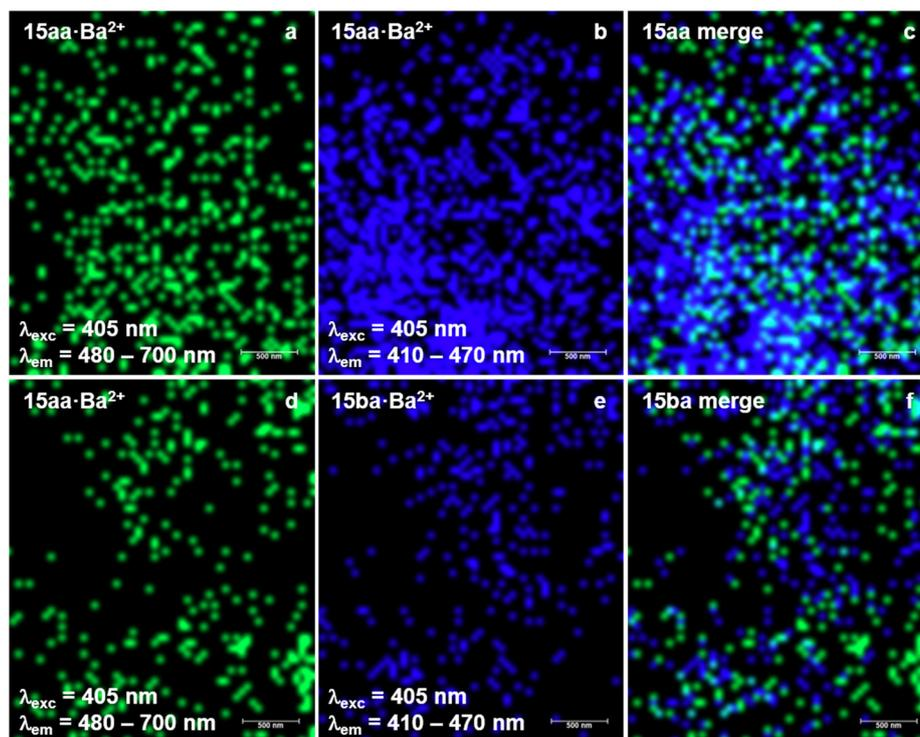
**Fig. 12** Confocal microscopy images of compounds **15aa** (panels a–c) and **15ba** (panels d–f) on ITO after sublimation of barium triflate, at the unbound and  $\text{Ba}^{2+}$ -bound channels (see Fig. 11, panels c and f), promising candidates for barium tagging.
