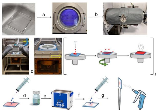
**Fig. 3** Protocol for the preparation of functionalized monolayers incorporating the fluorescent sensor on ITO. (a)  $\text{O}_2$ -activated plasma; (b) vacuum at  $60^\circ\text{C}$ ; (c) spin coating; (d) washing; (e) sonication; (f) washing; and (g) drying.
