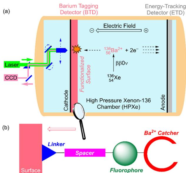
**Fig. 1** (a) Basic design of a BOLD (Barium atOm Light Detector) device for the neutrinoless double beta decay ( $\beta\beta 0\nu$ ) of  $^{136}\text{Xe}$  into  $^{136}\text{Ba}^{2+}$ . (b) Cartoon showing the components of a fluorescent indicator covalently anchored on an indium tin oxide (ITO) functionalized surface.
