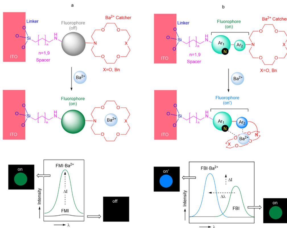
**Fig. 2** Fluorescent monocolor indicators (FMIs, a) and fluorescent bicolor indicators (FBIs, b) anchored to an indium tin oxide surface, as analyzed in the present work. The changes in intensity and/or wavelength in the emission spectra are highlighted.
