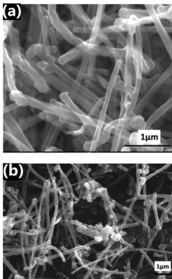
Fig. 12 SEM images of (a) pristine MWCNTs and (b) MWCNT:SnO<sub>2</sub> composites. This figure has been reproduced from ref. 174 with permission from Elsevier, copyright 2018.
