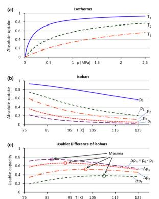
Fig. 5 Plots of absolute uptake and usable capacity of hydrogen against various temperatures and pressures showing: (a) typical type I adsorption isotherms plotted at various temperatures,  $T_1$ ,  $T_2$  and  $T_3$ . (b) Usable capacity when plotted at isobars for various pressures, Po, P1,  $P_2$ ,  $P_3$ , and  $P_4$  at different temperatures. (c) Isobars with the usable capacity as the change in absolute adsorption at difference in pressure ΔP. Reproduced with permission from ref. 96.
