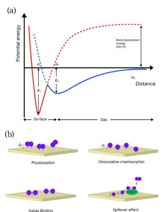
Fig. 1 (a) Potential energy curves for physisorbed and chemisorbed hydrogen as a function of distance d from the surface of the adsorbate. Adapted from ref. 17; (b) a schematic showing the different types of mechanisms for hydrogen adsorption on an adsorbate surface
