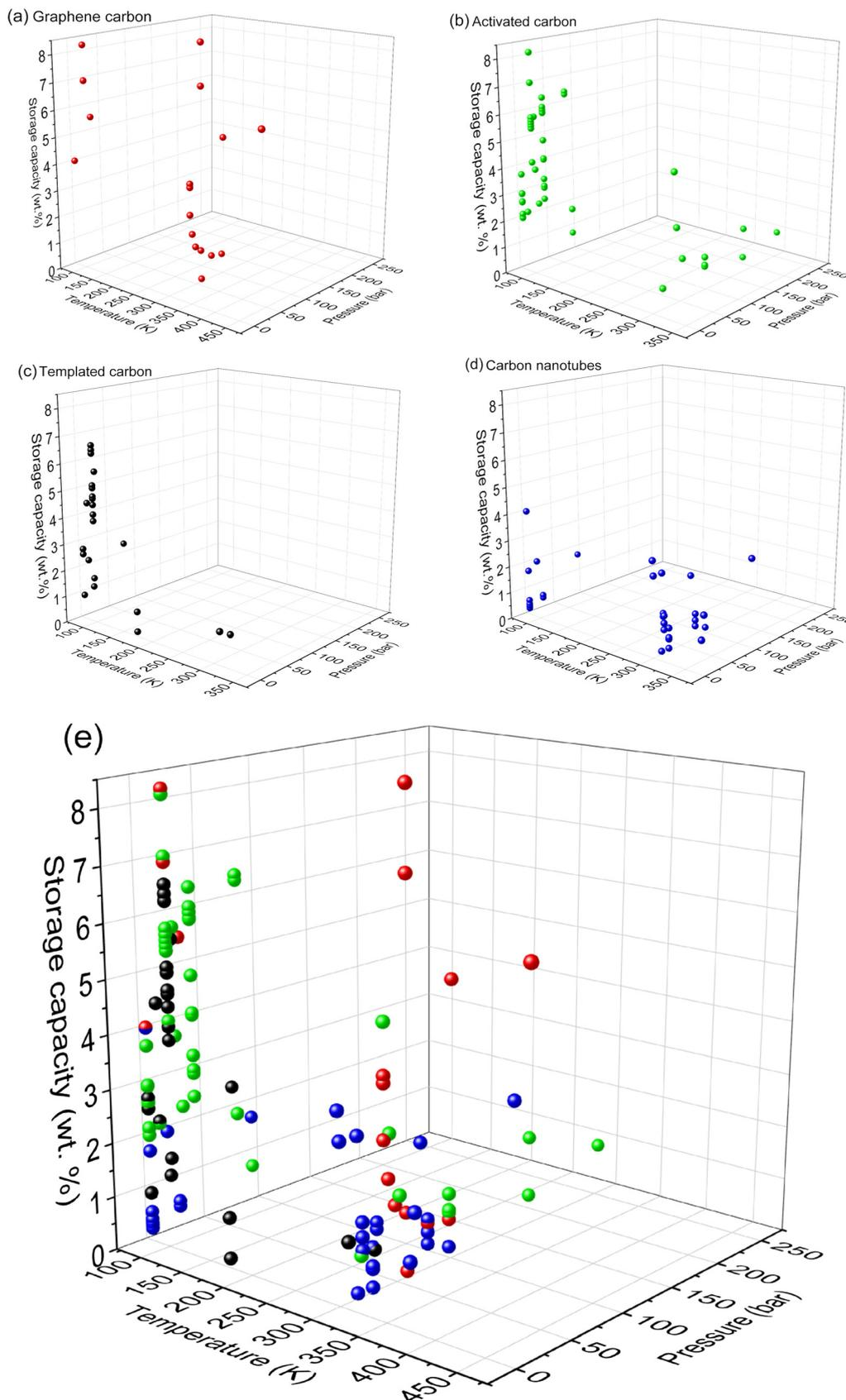
**Fig. 6** Scatter plot of temperature (K) and pressure (bar) versus excess storage capacity (wt%) for (a) graphene materials, (b) activated carbon, (c) template-derived carbons, and (d) carbon nanotubes taken from reported data. (e) Overlay of scatter plots (a)–(d). Plotted from the data reported in references listed in Table 3.
