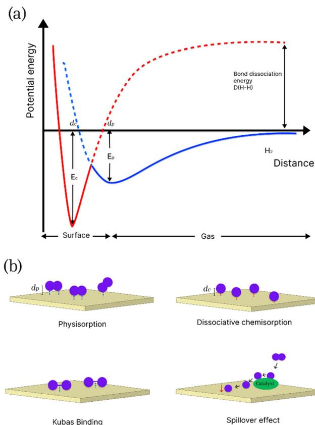
**Fig. 1** (a) Potential energy curves for physisorbed and chemisorbed hydrogen as a function of distance  $d$  from the surface of the adsorbate. Adapted from ref. 17; (b) a schematic showing the different types of mechanisms for hydrogen adsorption on an adsorbate surface.
