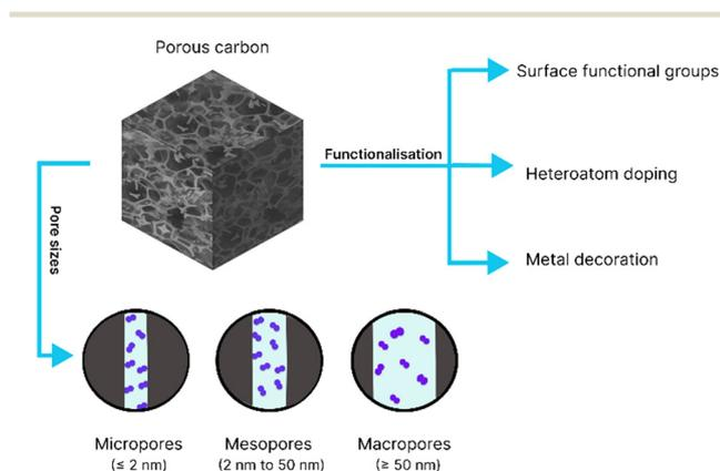
**Fig. 3** Schematic showing the structure property relationship of porous carbon, the pore size and types of functionalization, which are important factors in enhancing hydrogen uptake in carbon-based sorbents.
