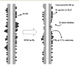
Fig. 11 Schematic showing the effect of the activation process on the structural morphology of CNTs. This figure has been reproduced from ref. 220 with permission from Elsevier, copyright 2007.
