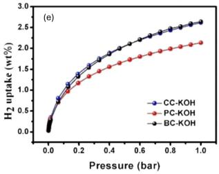
Fig. 14 SEM image of carbon derived from cornstalk (CC), after (a) thermal activation at 800 °C, (b) ZnCl<sub>2</sub> activation, (c) H<sub>3</sub>PO<sub>4</sub> activation and (d) KOH activation. (e) H2 adsorption for the KOH activated carbons derived from bagasse, cornstalk and pine powder shown. This figure has been reproduced from ref. 133 with permission from John Wiley and Sons, copyright 2020.
