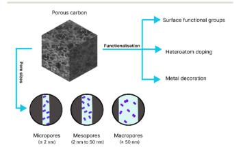
Fig. 3 Schematic showing the structure property relationship of porous carbon, the pore size and types of functionalization, which are important factors in enhancing hydrogen uptake in carbon-based sorbents
