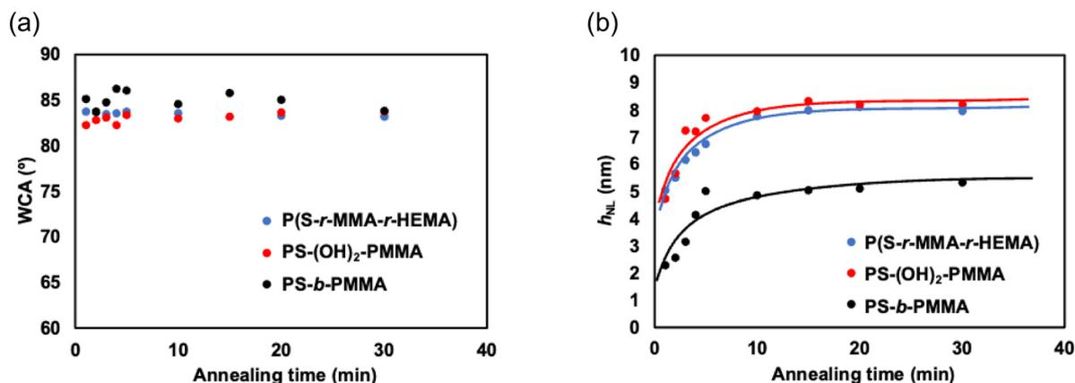
Fig. 3 (a) Water contact angles (WCAs) of the neutral layers formed by P(S-*r*-MMA-*r*-HEMA), PS-(OH)<sub>2</sub>-PMMA, and PS-*b*-PMMA annealed at 250 °C for different times. (b) Thicknesses of neutral layers ( $h_{\text{NL}}$ ) formed by P(S-*r*-MMA-*r*-HEMA), PS-(OH)<sub>2</sub>-PMMA, and PS-*b*-PMMA annealed at 250 °C for different times.
