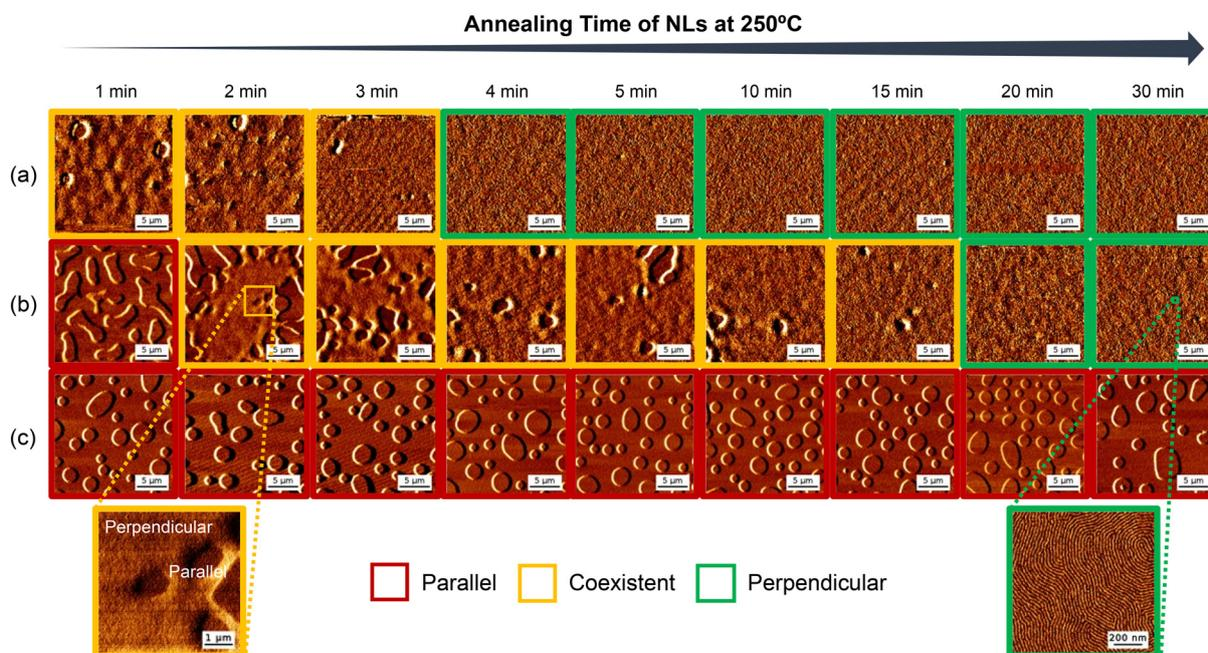
Fig. 2 AFM phase images (20 μm square) of PS-(OH)<sub>2</sub>-PMMA thin films (~30 nm) applied onto (a) P(S-r-MMA-r-HEMA) neutral layers, (b) PS-(OH)<sub>2</sub>-PMMA neutral layers, and (c) PS-*b*-PMMA neutral layers, which were annealed for various times from 1 to 30 minutes, accompanied by the magnified AFM phase images of coexistent orientation (5 μm square, bottom left) and perpendicular orientation (1 μm square, bottom right).
