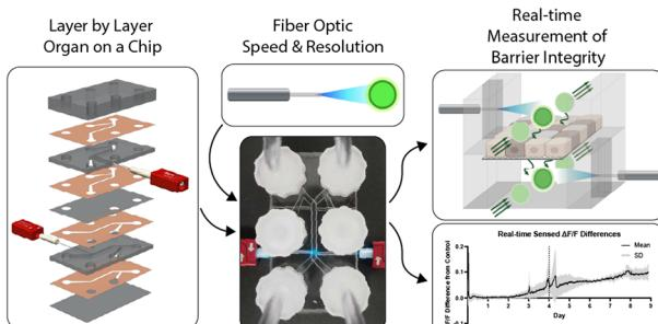
***In situ* monitoring of barrier function on-chip via automated, non-invasive luminescence sensing**
