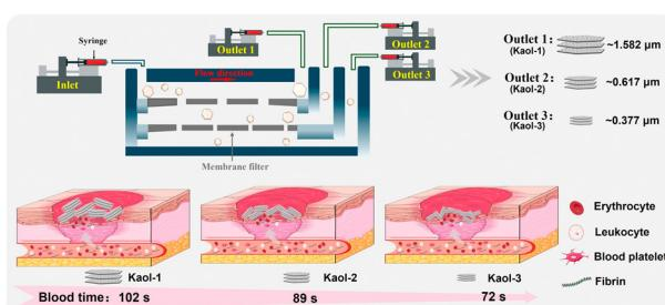
**Size-selective sorting of kaolinite micro/nanoflakes via microfluidic filtration for wound hemostasis**
