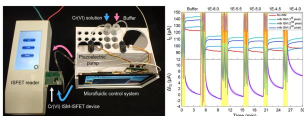
**Continuous and automatic hexavalent chromium sensing using an ion-selective membrane deposited ion-sensitive field-effect transistor device integrating a microfluidic control system**
