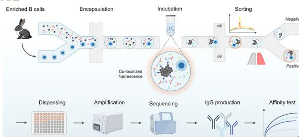
**High-throughput monoclonal antibody screening from immunized rabbits via droplet microfluidics**
