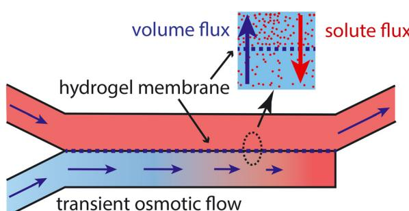
**Transient osmotic flows in a microfluidic channel: measurements of solute permeability and reflection coefficients of hydrogel membranes**
