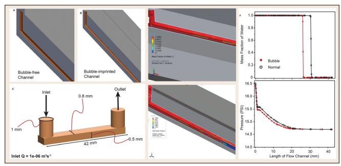
Fig. 6 Computational evaluation of the effect of channel-imprinted bubbles on flow characteristics. (A and B) 3D CAD models for computational simulation to study the effect of bubbles on fluid flow. (C) Internal dimensions of the flow channels of A and B. (D and E) Surface plot of A and B showing mass fraction of water in the fluidic channels. F shows XY plots of mass fraction of water (top) and pressure (bottom) resulting from bubble-free channel (black) and bubble-imprinted channel (red).
