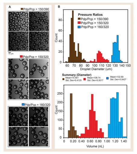
Fig. 7 A. Confocal micrographs showing droplets generated at varying driving pressure ratios. B. Histograms showing the distribution of C-top droplet volume (nL) and C-bottom droplet diameter (µm).
