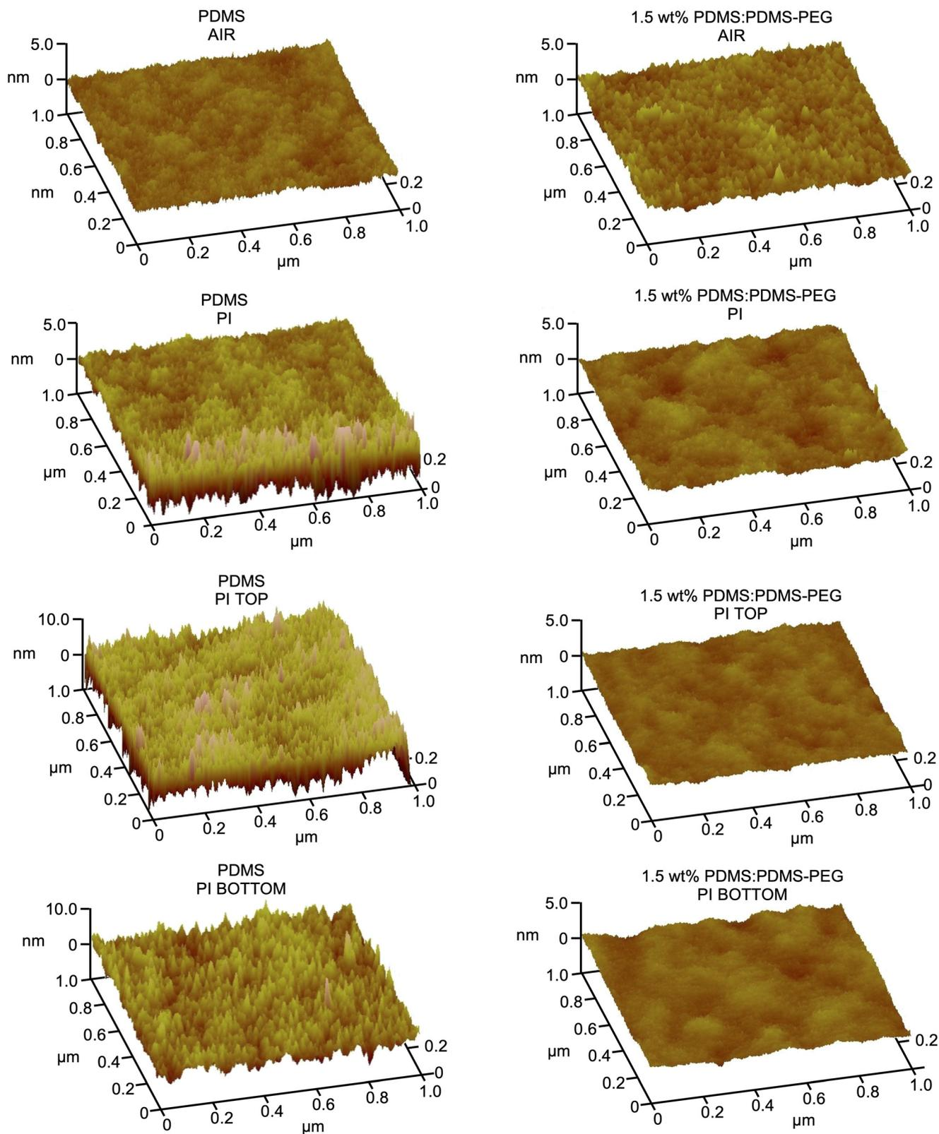
**Fig. 3** Surface characterization of PDMS and PDMS:PDMS-PEG films using AFM (tapping mode). Atomic force microscopy (AFM) images of pristine PDMS and 1.5 wt% PDMS:PDMS-PEG films were obtained to analyze the surface morphology under two fabrication configurations: AIR/PI and PI TOP/PI BOT.
