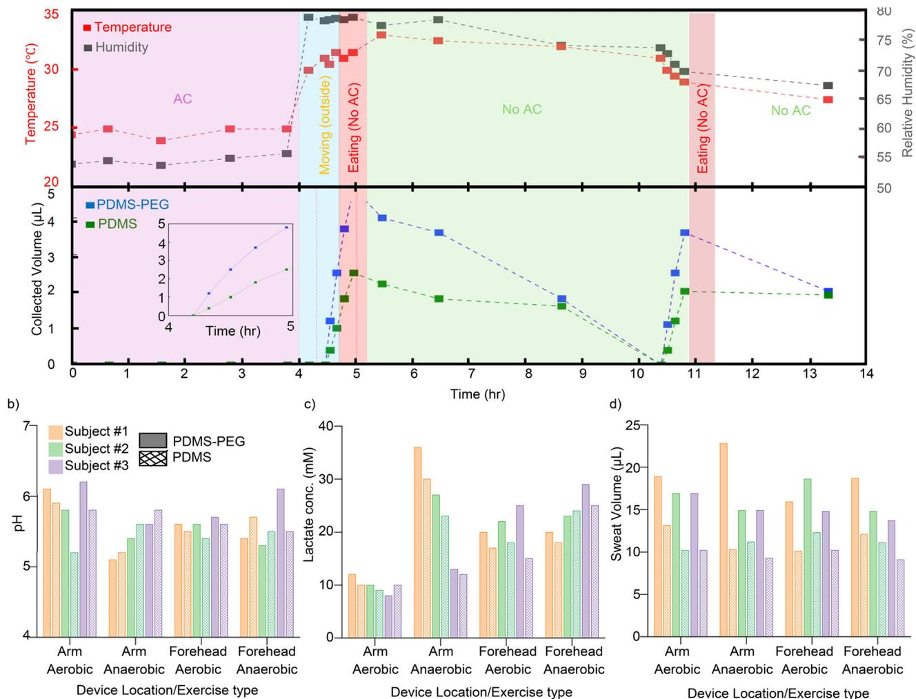
**Fig. 6** Feasibility study of the PDMS:PDMS-PEG microfluidic devices in human subjects. (a) Images from a half-day, non-exercise wear test showing the PDMS:PDMS-PEG and PDMS microfluidic devices applied to the forearm before and after sweat collection. (b–d) Results from an exercise-based study evaluating: (b) sweat pH, (c) lactate concentration, and (d) sweat volume collected using the PDMS:PDMS-PEG and PDMS devices.
