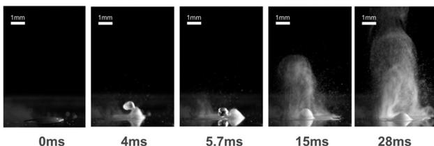
**Fig. 5** High-speed frames of a 1  $\mu\text{L}$  droplet on a 30 MHz SAW device with  $\text{O}_2$  plasma treatment, recorded at 0 ms, 4.0 ms, 5.7 ms, 15 ms, and 28 ms after SAW activation. In sharp contrast, the plasma-treated surface. The fluid is held in place which allows a larger sample volume to be sent to the MS compared to the untreated group.
