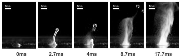
**Fig. 4** High-speed frames of a 1  $\mu\text{L}$  droplet on a 30 MHz SAW device without  $\text{O}_2$  plasma treatment recorded at 0 ms, 2.7 ms, 4.0 ms, 8.7 ms, and 17.7 ms after SAW activation. In the untreated case, SAW actuation quickly induces a strong ejection of several large satellite droplets in narrow jets (2.7–8.7 ms). These satellites are expelled at high velocity.
