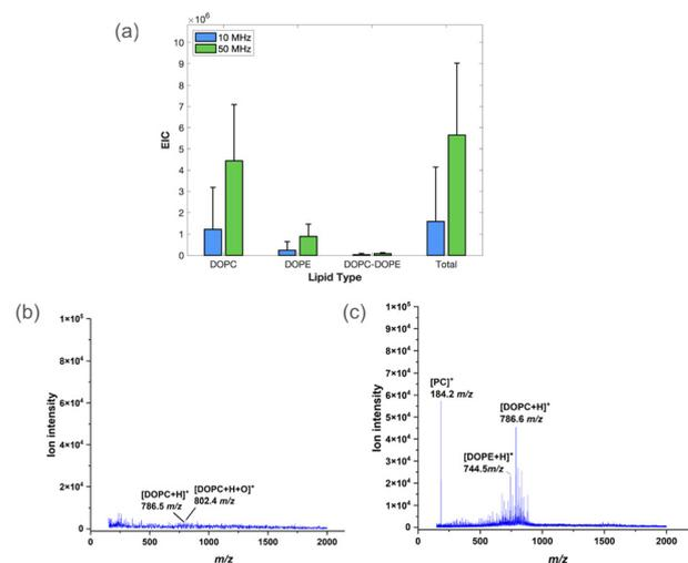
**Fig. 11** (a) Recovered EIC signals for individual lipid species and total signal at 10 MHz and 50 MHz. Quantified species include DOPC, DOPE, the heterodimer DOPC–DOPE, and the total recovered signal intensity. (b) and (c) Representative mass spectra showing ion intensity vs.  $m/z$  at 10 MHz and 50 MHz excitation, respectively. Enhanced signal intensity at 50 MHz reflects improved nebulization and lipid release efficiency.
