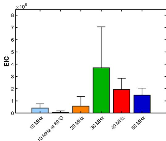
**Fig. 10** Extracted ion chromatogram (EIC) signal intensities for DOPC at varying SAW frequencies. Data include excitation at 10 MHz, 10 MHz with elevated temperature (60 °C), and higher frequencies up to 50 MHz. Increased EIC at 30–50 MHz indicates more efficient lipid nebulization at higher acoustic frequencies.
