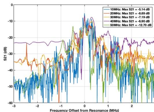
**Fig. 2**  $S_{21}$  (dB) as a function of normalized frequency offset from resonance.
