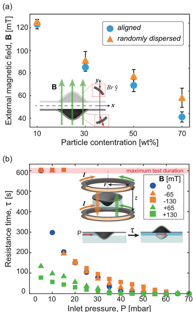
**Fig. 4** (a) An external magnetic field is required to actuate the valve, depending on particle concentration and alignment. Valves with higher remanent magnetization exhibit higher actuation thresholds. (b) Resistance time under constant inlet pressure as a function of applied current. Negative currents (orange) enhance valve sealing, while positive currents (green) promote opening.
