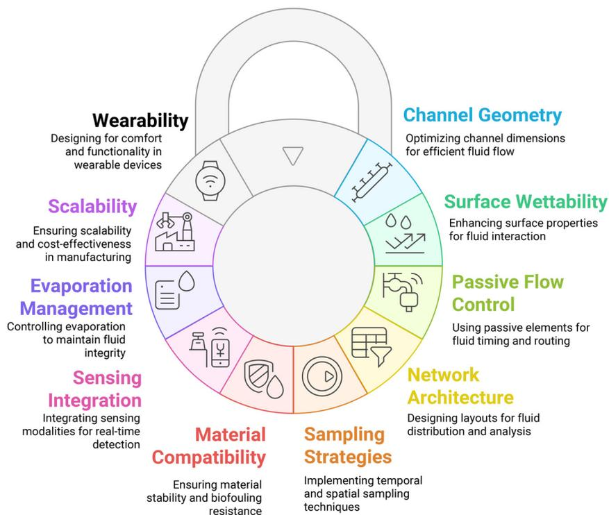
**Fig. 3** Key design principles for wearable capillary microfluidic systems ensuring efficient fluid handling, biochemical sensing, material compatibility, and user comfort. Integration of suitable materials, optimized channel layout, and sensor interfaces enables robust, autonomous operation for on-body and point-of-care applications.
