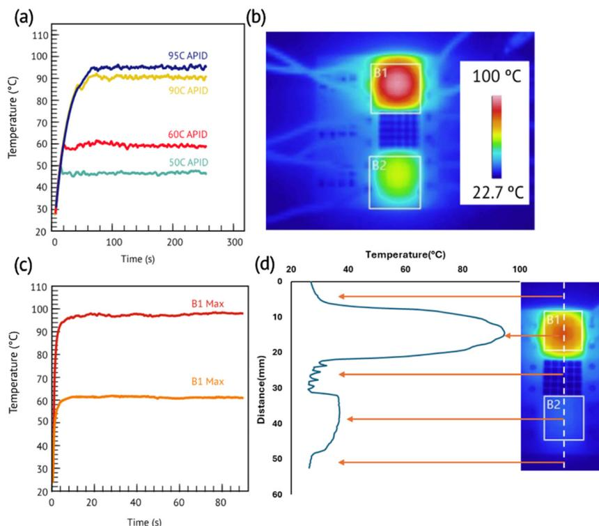
**Fig. 4** Heater temperature control with the aid of APID controller. (a) The heater temperature stabilization over time with APID set at 50 °C, 60 °C, 90 °C, and 95 °C, (b) two adjacent heaters heating at different temperatures, (c) the temperature stabilization of the two adjacent heaters, (d) the temperature distribution along the line containing two heaters at different temperature at 37 °C and 95 °C.
