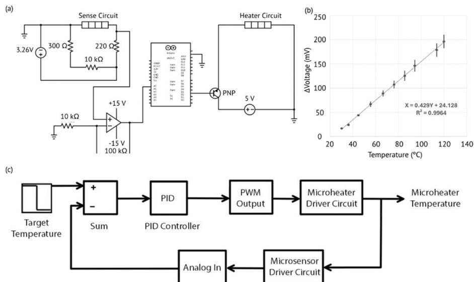
**Fig. 3** Heating-sensing controller system consisting of (a) micro-sensor resistive temperature detection circuit in bridge configuration with one step amplification and PWM heater circuit, (b) calibration curve of the micro-sensor, and (c) closed-loop control with PID controller in the sense circuit. The sensor calibration curve shows a linear regression fit between the applied voltage and the corresponding output temperature of the sensor.
