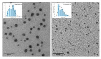
**Fig. 10** TEM images of AgNPs synthesized at a total flow rate of (left) 5 mL min<sup>-1</sup> and (right) 7 mL min<sup>-1</sup>. Size distribution histogram for each image are shown in insets.
