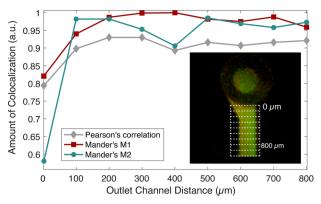
Fig. 7 PCC and MCC of fluorescence image of mixing in the microturbine at steady state. ROI down the outlet channel is depicted within the inset where each box represents a 100  $\mu$ m analysis area.
