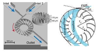
**Fig. 1** (Left) 3D rendering of the microturbine mixer with perspective view of rotor (inset). (Right) Drawing of the fluid flow profile through the mixer depicting entrained and crossflow paths.
