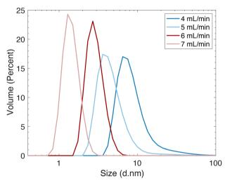
**Fig. 9** (Top) AgNP volume distributions for particles synthesized within a microturbine. (Bottom) DLS size distributions depicting the influence on particle size and flow rate.
