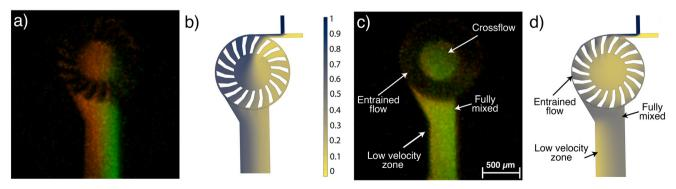
Fig. 6 Mixing profiles of (a) experimental and (b) simulated fluids, showing lamination for stationary rotor. (c) Merged channels of steady state flow (7 mL min<sup>-1</sup> total, rotor spinning) and (d) simulated. The fluorescence image resolution is approximately 3.6 μm per pixel.
