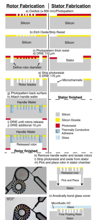
Fig. 2 Abbreviated fabrication process for microturbine mixer.
