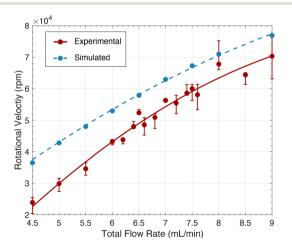
Fig. 5 Experimentally and computationally determined (COMSOL Multiphysics) rotational velocities as a function of flow rate. Experimental data is plotted as average velocity of 5 runs: error bars represent range of values.
