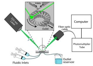
Fig. 4 Diagram of rotational velocity measurement set-up
