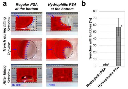
Fig. 3 A circular trench of 3 mm of diameter during and after filling it with red colorant. a) On the left, images of the filling using regular PSA in the bottom of the trench, and on the right using hydrophilic PSA. b) Bubble formation in devices with hydrophilic and hydrophobic pressuresensitive adhesives (PSA) at the bottom of the trenches. N = 150 trenches from three devices. Error is S.D. Different letters (a and b) indicate significant statistical difference (p < 0.005, z-test).
