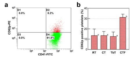
Fig. 6 Platelets activation assay. a) Representative result of flow cytometry showing the total platelets (D2 and D4) and the activated platelets (D2). b) Summary of the platelets activation results for the rectangular (RT), circular (CT) and two big (TbT) trenches devices along with the centrifugation method (CTF). Error is S.D. N = 3. Different letters (a and b) indicate significant statistical difference (p < 0.05, t-test).
