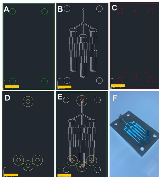
**Fig. 2** Kappa( $\kappa$ )Chip layer schematics. A. Bottom substrate for hydrophobin–polymer interaction tests. B. Adhesive/channel layer to define internal shear stresses. Three identical units containing eight shear stress tests. C. Top cover (PMMA) design. D. Double-sided adhesives for connecting microfluidic interfacing parts. E. Combined schematic of all layers. F. Fully assembled kappa( $\kappa$ )Chip. Yellow scale bar is 10 mm.
