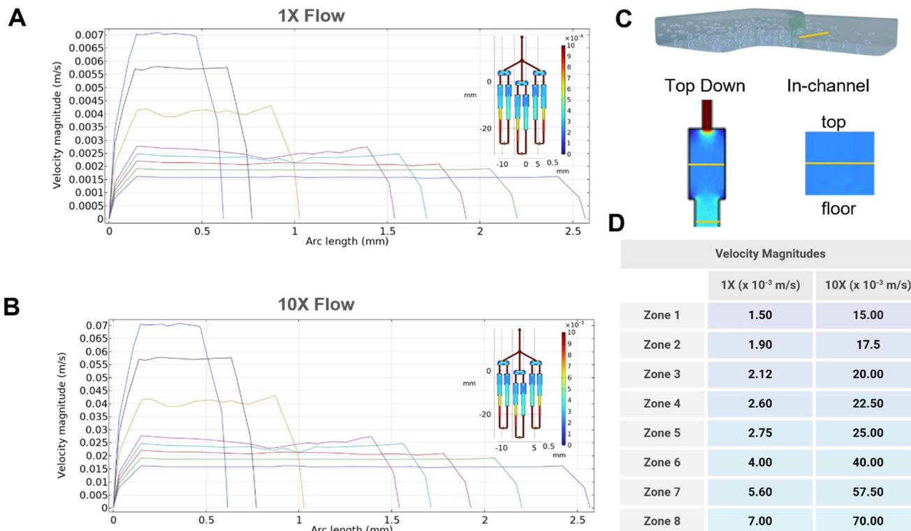
**Fig. 4** COMSOL simulation results demonstrating decreases in velocity magnitude as channel width increases. A. 1 $\times$  Flow pattern using the final kappa( $\kappa$ )Chip version. B. 10 $\times$  Flow pattern using the final kappa( $\kappa$ )Chip version. C. Arc length visual representation. Arc length in yellow. D. Velocity magnitudes extracted from A and B.
