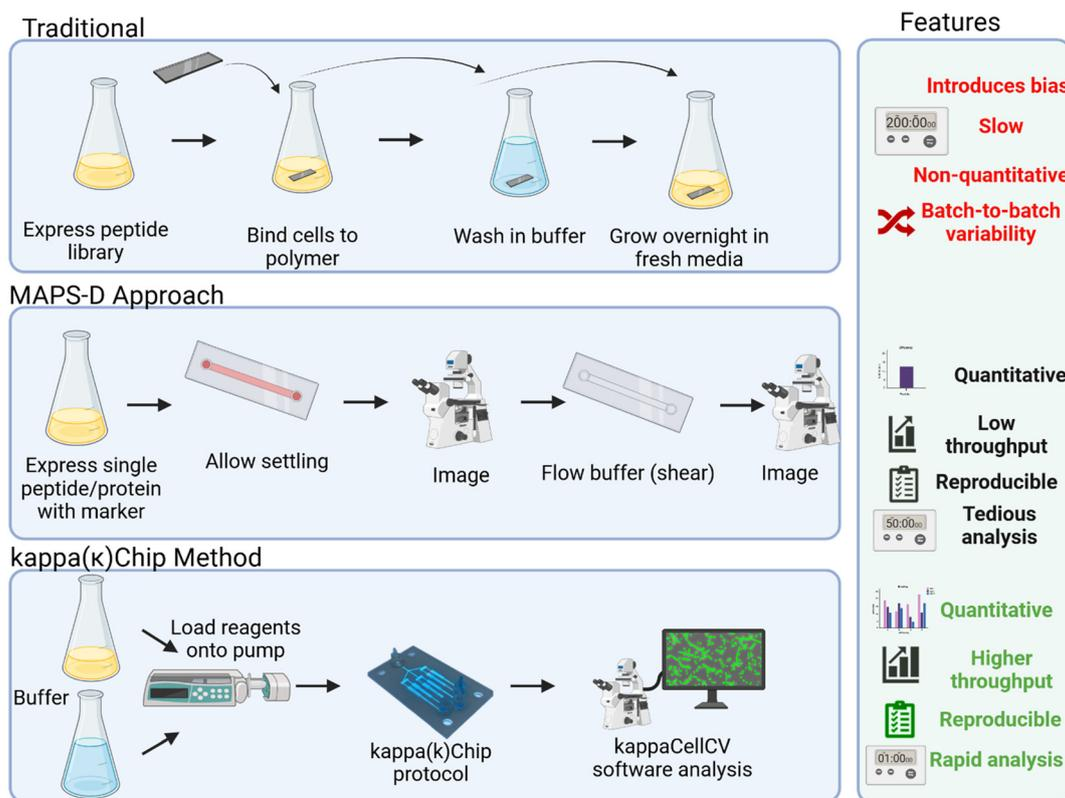
Fig. 1 Simplified workflow for kappa( $\kappa$ )Chip compared to a traditional method and the MAPS-D (publication forthcoming) approach also developed by DEVCOM Army Research Laboratory. Benefits and features are demonstrated in the features sidebar. MAPS-D: Microfluidic Assessment of Adhesion by Surface Display (publication forthcoming).
