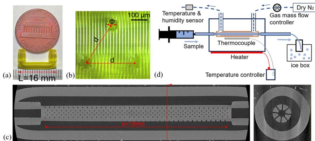
**Fig. 2** (a) Photograph of the fabricated device next to a one cent coin. (b) Photograph of the inner tube showing the micro-pores under a microscope. (c) CT images displaying both the front (left) and cross-section (right) views of the 50  $\mu\text{m}$  micro-pore evaporator, highlighting the micro-pores and the channel within. The scale bar at the top right of the front view applies to both images. (d) Schematic of the experimental system for evaporator–concentrator testing.
