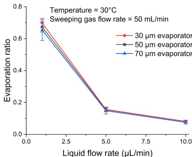
**Fig. 7** Deionized water evaporation *versus* liquid flow rate from 1 to 10 μL min<sup>-1</sup> for three different pore diameters under the condition of 30 °C and 50 mL min<sup>-1</sup> of sweeping gas flow rate.
