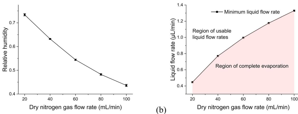
Fig. 4 Experimentally determined (a) relative humidity and (b) liquid flow rate for various dry nitrogen gas flow rates range from 20 to  $100 \text{ mL min}^{-1}$  at  $30 \text{ }^\circ\text{C}$ . The liquid flow rate is  $2 \mu\text{L min}^{-1}$ .
