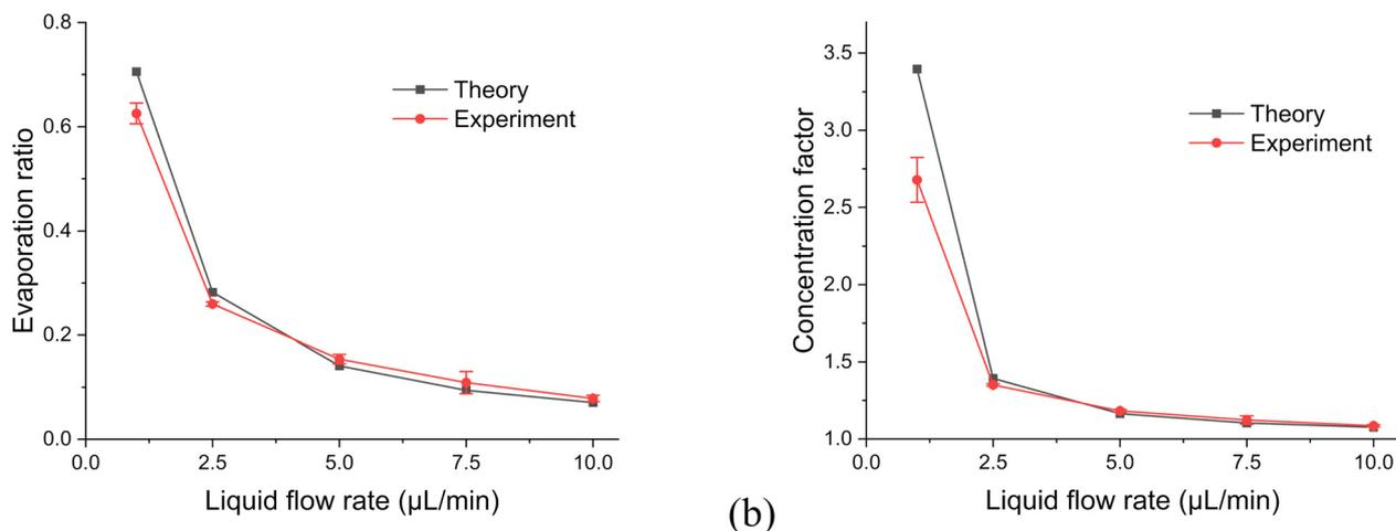
**Fig. 6** Deionized water evaporation and corresponding concentration factors under experimental conditions of 30 °C temperature and a 50 mL min<sup>-1</sup> dry nitrogen gas flow rate. (a) Evaporation ratio *versus* liquid flow rate from 1 to 10 μL min<sup>-1</sup>. (b) Concentration factor *versus* liquid flow rate from 1 to 10 μL min<sup>-1</sup>.
