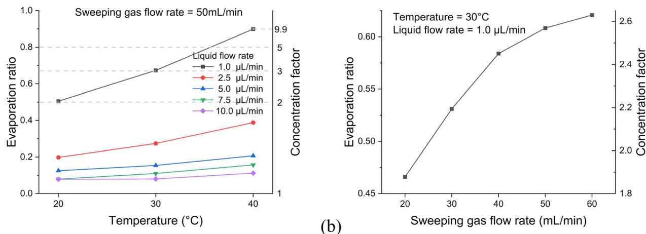
Fig. 5 (a) Evaporation ratio and concentration factor as a function of temperature for various liquid flow rates, with a constant sweeping gas flow rate of 50 mL min<sup>-1</sup>. (b) Evaporation ratio and concentration factor for different sweeping gas flow rates, with a constant temperature of 30 °C and liquid flow rate of 1.0 μL min<sup>-1</sup>.
