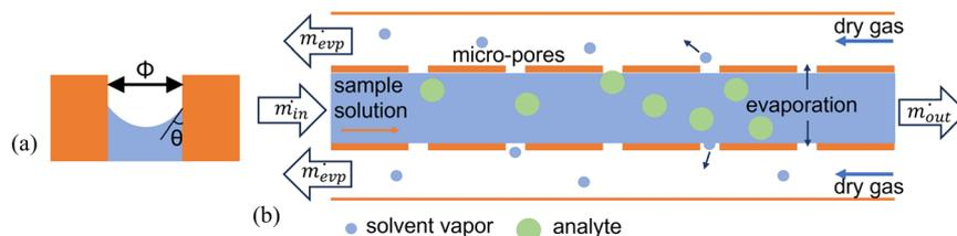
Fig. 3 (a) Schematic of capillary-driven liquid retention in a single hydrophilic micro-pore.  $\Phi$  represents the diameter of the micro-pore, and  $\theta$  represents the contact angle. (b) General schematic of a micro-pore evaporator.
