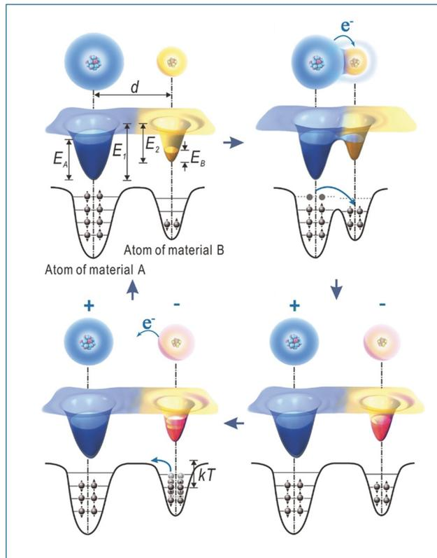
Fig. 9 Electron-cloud-potential-well model. Reproduced with permission.<sup>199</sup> Copyright 2018, Wiley-VCH GmbH.
