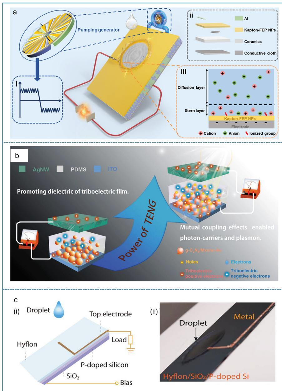
**Fig. 11** a) Externally charge-pumped liquid–solid TENG. Reproduced with permission.<sup>222</sup> Copyright 2024, Wiley-VCH GmbH. b) Enhance TENG performance through charge trapping facilitated by photon-induced carrier generation.<sup>223</sup> Copyright 2021, Wiley-VCH GmbH. c) Field-effect-enhanced droplet electricity generator.<sup>224</sup> Copyright 2023, Wiley-VCH GmbH.
