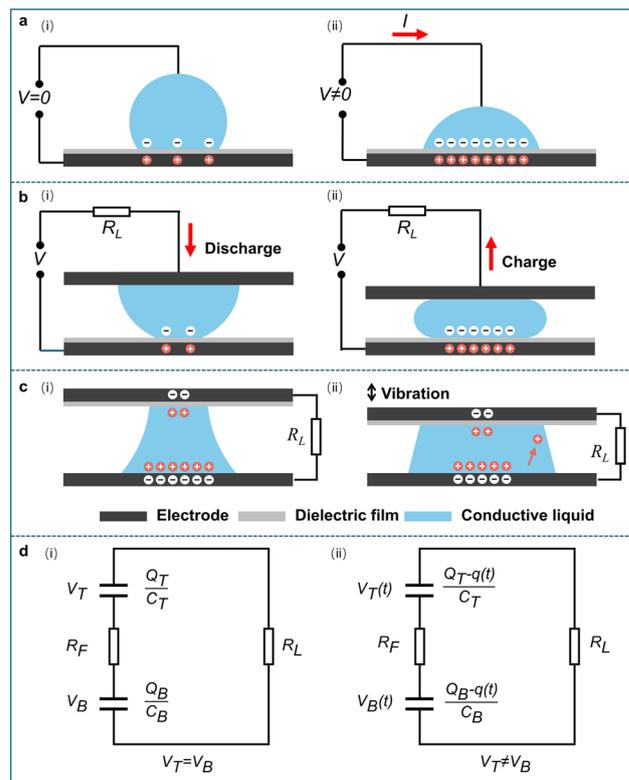
**Fig. 3** Basic working principles and equivalent circuit diagram. a) Working principle of the EWOD process. (i) No external voltage applied between the metal and the electrolyte solution; (ii) external voltage applied between the metal and the electrolyte solution. b) Working principle of the REWOD process. c) Working principle of the water bridge REWOD process. d) Equivalent circuit diagram of the water bridge REWOD process.
