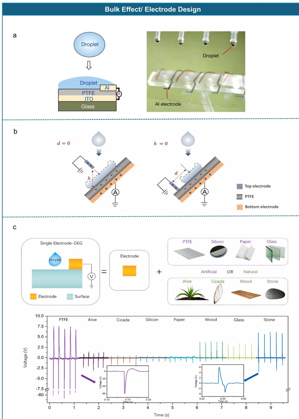
**Fig. 12** a) First bulk effect droplet-based electricity generator. Reproduced with permission.<sup>90</sup> Copyright 2020, Springer Nature. b) Transistor-like design for droplet energy harvesting. Reproduced with permission.<sup>234</sup> Copyright 2023, Elsevier. c) Universal single-electrode configuration. Reproduced with permission.<sup>235</sup> Copyright 2021, Elsevier.
