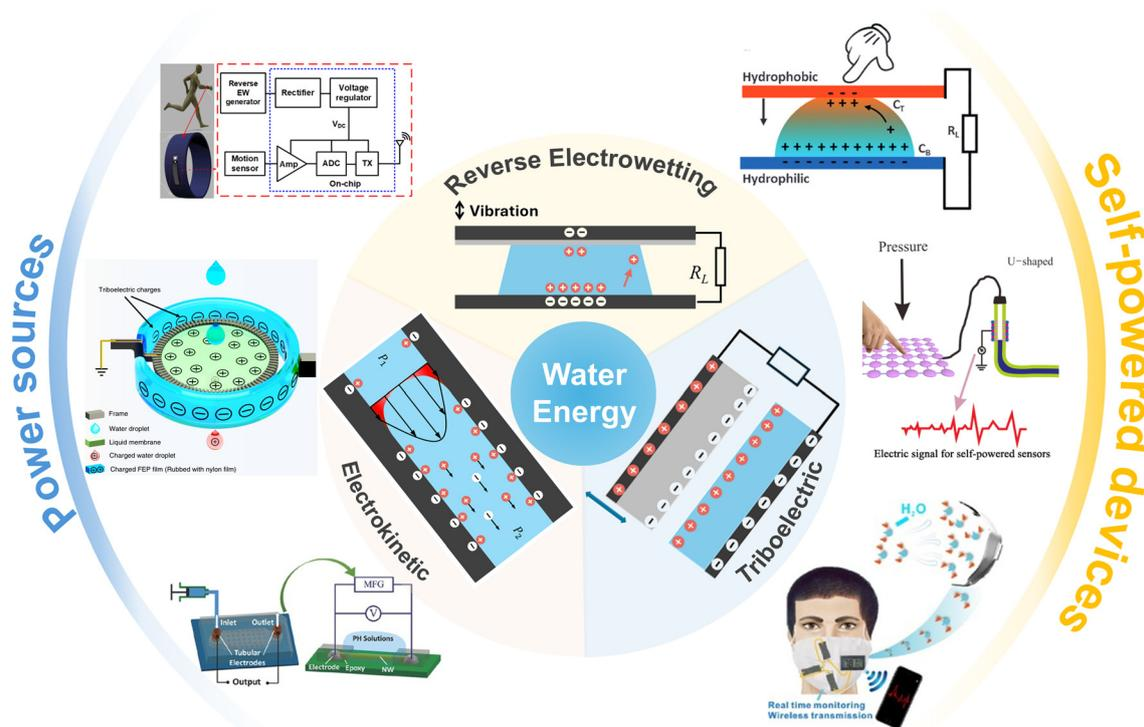
Fig. 1 Summary of the working principles and applications of REWOD, TENG, and EKEC. Reproduced with permission.<sup>26</sup> Copyright 2020, IEEE. Reproduced with permission.<sup>27</sup> Copyright 2016, Wiley. Reproduced with permission.<sup>28</sup> Copyright 2017, Elsevier. Reproduced with permission.<sup>29</sup> Copyright 2019, Springer Nature. Reproduced with permission.<sup>31</sup> Copyright 2015, Wiley. Reproduced with permission.<sup>30</sup> Copyright 2023, Elsevier.
