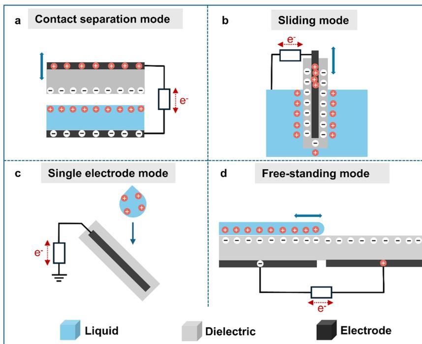
**Fig. 8** Basic modes of operation. (a) Contact-separation mode, (b) sliding mode, (c) single-electrode mode and (d) free-standing mode TENGs, respectively. Blue bidirectional arrows indicate the periodic mechanical motion. Red bidirectional arrows labeled “e<sup>-</sup>” represent the cyclic electron flow in the external circuit that changes direction during different phases of the mechanical cycle.
