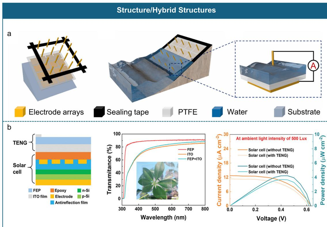
Fig. 14 a) Wave energy harvester utilizing a liquid-solid TENG planar array. Reproduced with permission.<sup>244</sup> Copyright 2021, Elsevier. b) Stacked configuration of a liquid-solid TENG and solar cell. Reproduced with permission.<sup>245</sup> Copyright 2023, Wiley-VCH GmbH.
