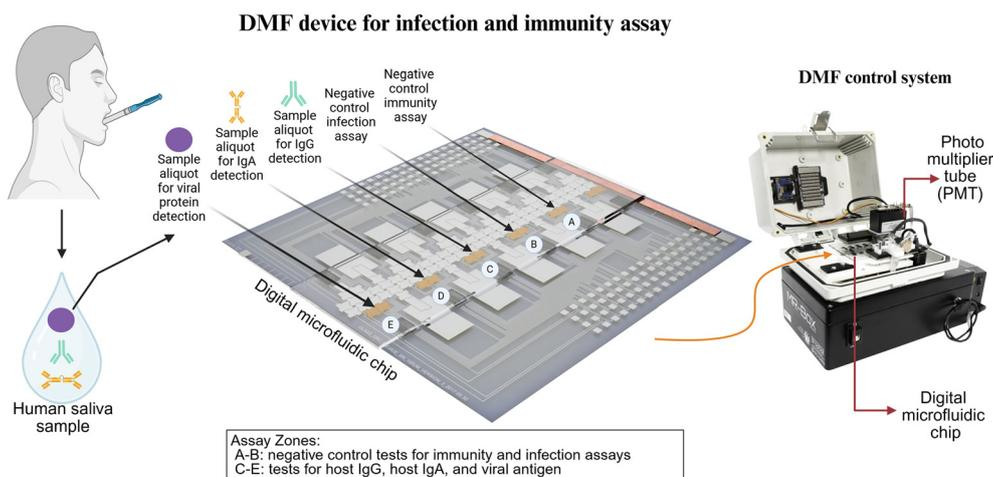
**Fig. 1** Digital microfluidic test for infection and immunity status. Schematics (left) illustrating bead-based immunoassays on a digital microfluidic for multiplexed, quantitative detection of negative controls (A and B), host IgG and IgA (C and D), and viral antigen (E) in saliva. Photo (right) of the DMF control system used to automate the tests.
