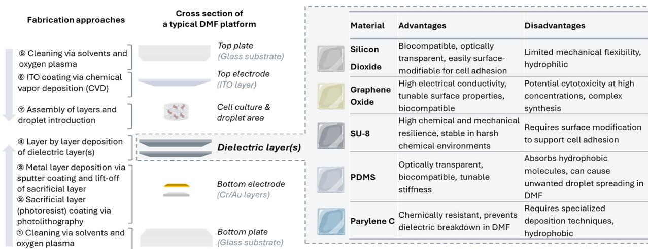
**Fig. 3** Cross section of a typical passive glass DMF platform (middle) including the layer composition. General fabrication workflow including example approaches are listed on the left, and a comparison between advantages and disadvantages of the commonly used dielectric materials in DMF platforms for cell culturing are shown on the right.
