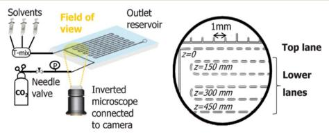
Fig. 2 Schematic representation of the experimental setup with the field of view. In the field of view, the top lane shows bubble shrinkage due to absorption; the lower lanes show slow expansion due to pressure drop.<sup>29</sup>
