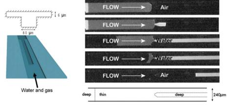
Fig. 18 [Left] Microfluidic gas-liquid phase separation for  $CO_2$  measurement. Schematic of the microchannel design, featuring deep and thin regions for controlled phase separation. [Right] Experimental images showing sequential air and water flow, demonstrating effective gas isolation for inline  $CO_2$  analysis with infrared absorption spectroscopy.<sup>86</sup>
