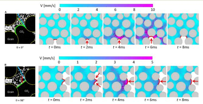
Fig. 28 [Top] Evolution of velocity fields during a Haines jump event in drainage. [Bottom] Evolution of velocity fields during a cooperative filling event in weak imbibition.<sup>167</sup>
