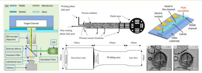
Fig. 24 [Left] A schematic diagram illustrating the on-chip pressure sensor enabled by astigmatic particle tracking. [87] [Middle] Micromodel with integrated fiber-optical pressure sensors. [88] [Right] 3D sketch of the microfluidic chip with integrated SIP sensors and sample results of calcite dissolution. [86]
