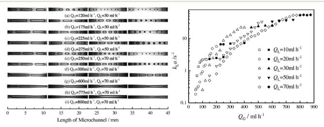
Fig. 11 [Left] Experimental image of gas-liquid flow at different flow rates (from a to i). [Right] The calculated volumetric mass transfer coefficient  $(k_{La})$  for different flow rates.<sup>58</sup>
