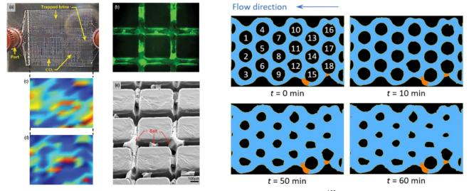
Fig. 29 [Left] Experiments of salt precipitation in the regular grid-like microfluidic network in PMMA.<sup>169</sup> [Right] Evolution of the calcite grains over time, subject to dissolution by HCl. The dissolution rate is shown to be strongly dependent on the pore flow and the presence of gas bubbles. 184
