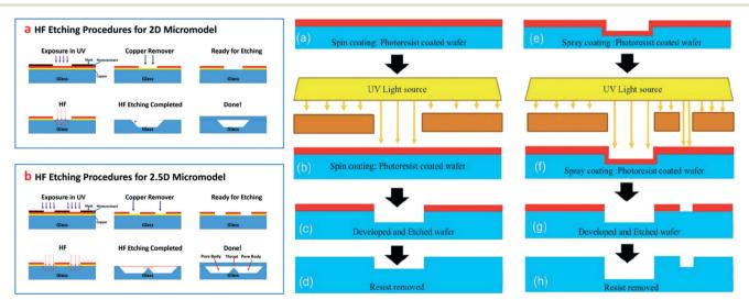
Fig. 22 [Left] Fabrication steps of a 2.5D micromodel.<sup>165</sup> [Right] Fabrication steps of a dual-porosity dual-depth micromodel.<sup>179</sup>
