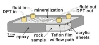
Fig. 19 [Left] The schematic of carbon mineralization occurring in different zones of a fractured mafic/ultramafic rock. [Right] The schematic showing a microfluidic model system used to investigate carbon mineralization in a fracture.<sup>111</sup>
