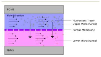
Fig. 9 Schematic representation of convection-diffusion mass transport in a microfluidic device. Molecules from the highconcentration stream (purple) diffuse into the low-concentration stream (pink) while convecting downstream, illustrating the simultaneous influence of advection and diffusion on mass transfer within the microchannel.52
