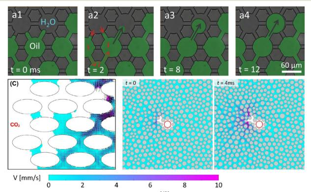
Fig. 26 [Top] High-speed images of a Haines jump event at  $Ca = 3.4 \times 10^{-6}$ . [Bottom] Velocity vector fields during a Haines jump event in linear drainage and radial drainage. <sup>146,167</sup>
