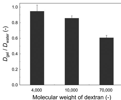
**Fig. 4** Relative diffusion coefficients ( $D_{\text{gel}}/D_{\text{water}}$ ) of FITC-dextran (MW: 4000, 10 000 and 70 000 Da) in Ca-alginate hydrogel, normalized by their diffusion coefficients in water. Diffusion coefficients were determined using FRAP. Data represent the mean  $\pm$  S.D. ( $n = 5$ , independent measurements).
