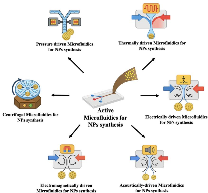
**Fig. 13** Schematic description of NP generation in different passive and active microfluidic devices.
