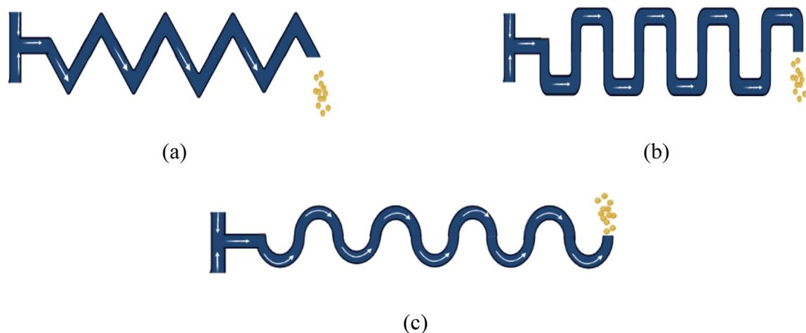
Fig. 10 Schematic diagram of different shaped microchannels for better mixing a) zig-zag b) square c) serpentine shaped microchannels.
