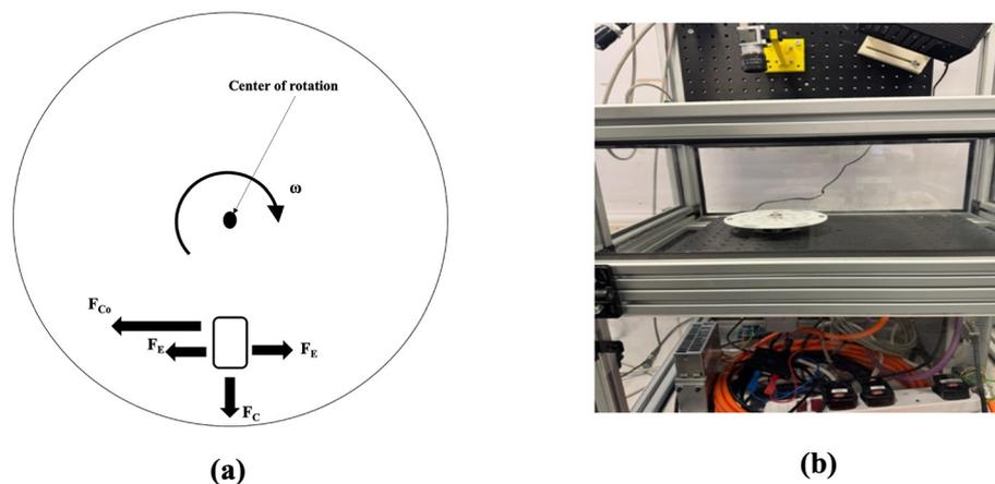
**Fig. 12** a) Pseudo-forces acting in centrifugal microfluidics. Centrifugal force ( $F_C$ ) always acts radially outward, the Coriolis force ( $F_{Co}$ ) acts perpendicular to both  $\omega$  and the fluid velocity and the Euler force ( $F_E$ ) is proportional to the angular acceleration. b) Centrifugal microfluidic system.
