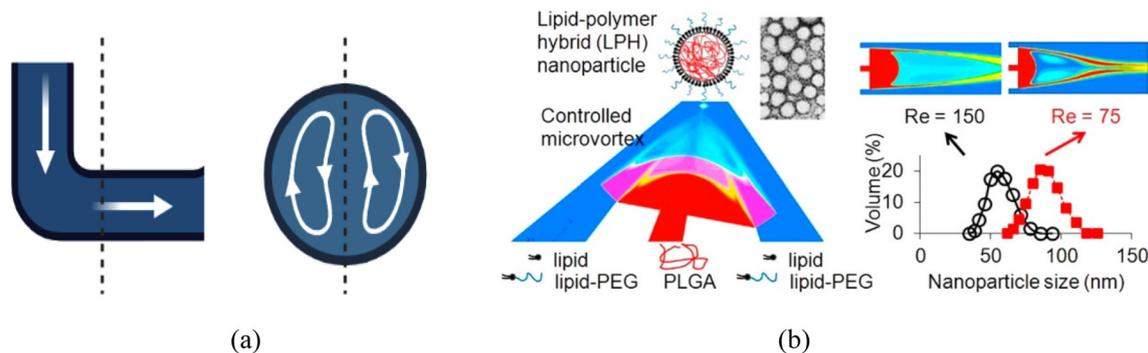
Fig. 9 a) Schematic diagram of secondary flow in a microchannel; b) schematic cross-sectional view of a three-inlet microfluidic system used for the synthesis of lipid-polymer hybrid NPs with the help of microvortices adapted with permission from<sup>273</sup> Copyright (2012) American Chemical Society.
