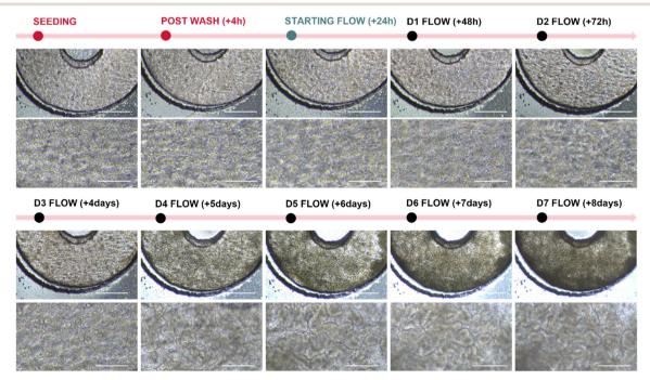
Fig. 3 3DP-μGut maturation. Phase contrast imaging of the Caco-2 maturation inside the 3DP-μGut devices during one week under flow conditions, n = 4. Top images: bar = 500  $\mu$ m, bottom images: bar = 250  $\mu$ m.
