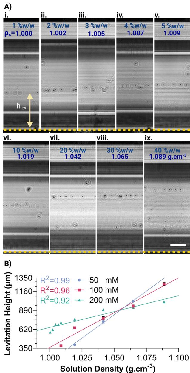
Fig. 4 Density measurements in the MagSity platform. A. Reconstructed images of microparticles spiked in different concentrations (0–50%) of glycerol, resulting in different solution densities (i–ix). 200 mM  $Gd^{3+}$  was used in the experiments.  $h_{lev}$  is the levitation height of the particle to the bottom magnet. Scale bar, 500  $\mu$ m. B. Density calibration curve for 50–200 mM  $Gd^{3+}$ .
