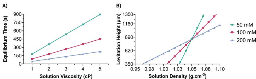
Fig. 2 Simulation results. Simulated A. equilibrium and B. levitation heights of microparticles in solutions with different viscosities and densities. In the simulations, 1.05  $\text{g cm}^{-3}$  microparticles with a diameter of 15  $\mu\text{m}$  spiked in 50–200 mM  $\text{Gd}^{3+}$  were utilized.
