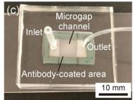
Fig. 3 (a) SEM image showing the microcone structure prepared by T-NIL on a PC sheet. (b) Fluorescence microscopic image showing the boundary between the coated and non-coated areas with fluorescence-labeled antibody. (c) Photograph of the assembled microfluidic device with the microgap channel.
