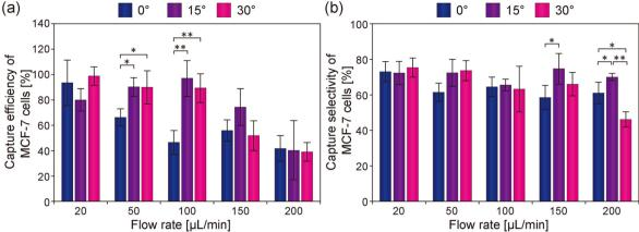
Fig. 5 Effects of the flow rate and the orientation angle of the microcone array on (a) capture efficiency and (b) selectivity of MCF-7 cells. Each data shows the mean  $\pm$  SD of 4 experimental results. \*p < 0.05, \*\*p < 0.01.
