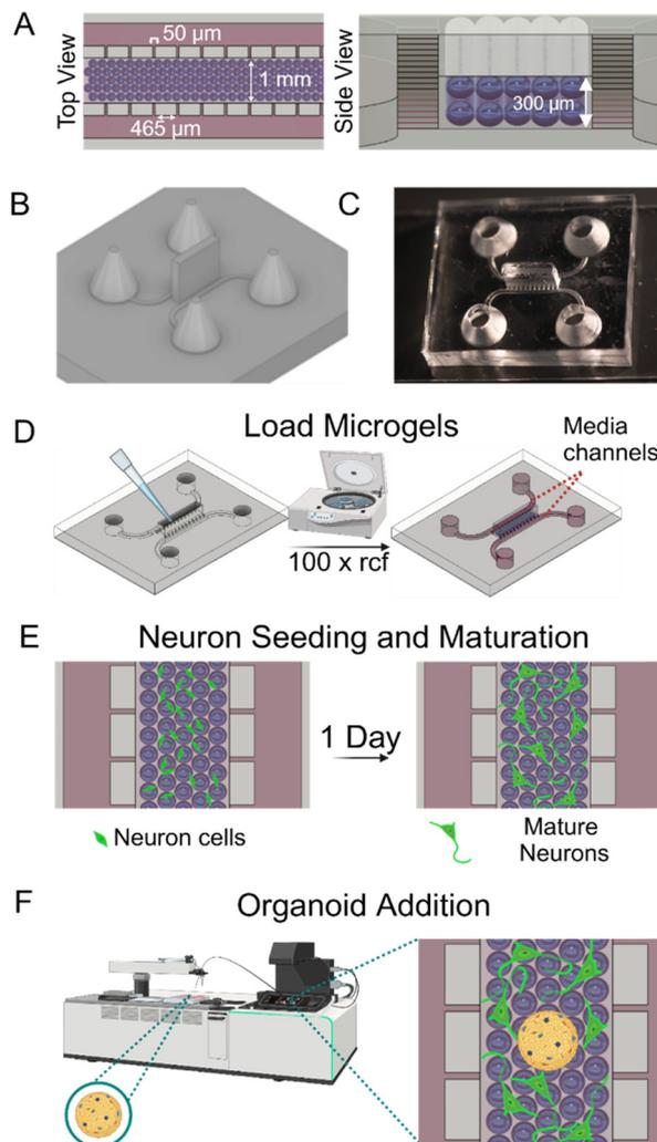
**Fig. 1** Device design and schematics. (A) Schematic of top and side views of the device loaded with microgels. (B) CAD drawing of the negative master-mold. (C) Photograph of the device. (D–F) Schematic of how microgels are loaded into the device, neurons are cultured, and organoids are added to the device.
