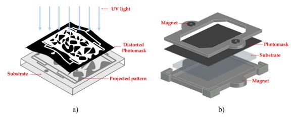
Fig. 12 (a) Encountered pattern distortion issue by holding photomask with tape. (b) CAD image of the newly designed wafer holder.
