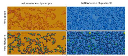
Fig. 11 Pore network of both cropped permeability chips: limestone pattern (left) and sandstone pattern (right).
