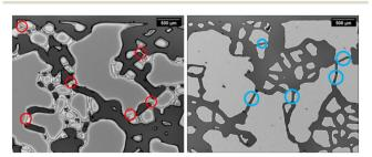
Fig. 13 The resulting patterns from mask alignment with tape (left) and with support (right). Red circles indicate areas that were not transferred due to poor UV incidence on the photoresist layer (distorted mask).
