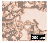
Fig. 8 Superimposed image of rescaled pattern (light color regions) and microscope images (dark contours) from (left) cropped limestone pattern and (right) the extra original limestone pattern, both chips were etched at the same conditions.
