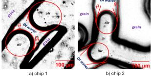
Fig. 9 Superimposed image of marked references for contact angle (red) and microscope images during water injection from (a) cropped limestone pattern and (b) the extra original limestone pattern. Contact angles show water-wet behavior.
