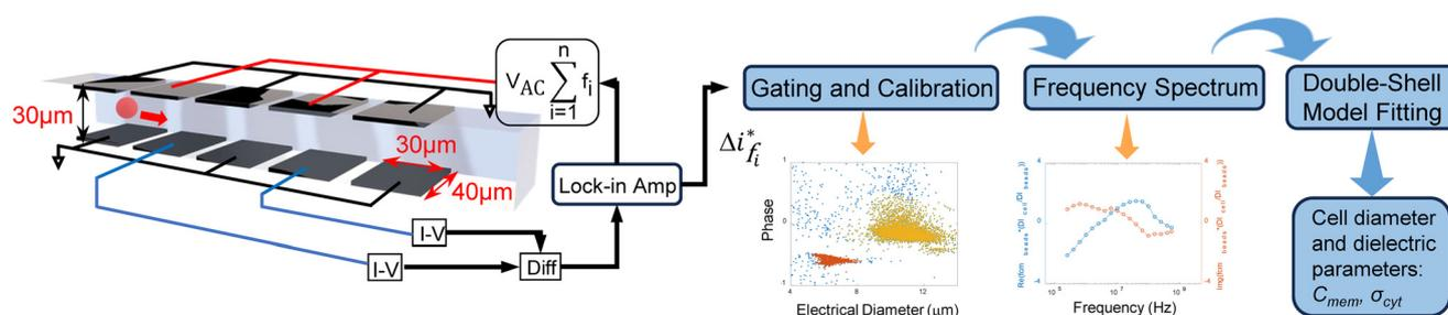
**Fig. 2** System overview and measurement principle. Cells suspended in saline flow along the microchannel where microelectrodes measure the differential current at different frequencies ranging from 250 kHz to 550 MHz. After gating and calibration, the frequency spectrum was fitted to the double-shell model to give cell diameter and cell dielectric parameters (membrane capacitance:  $C_{mem}$ , cytoplasm conductivity:  $\sigma_{cyt}$ ).
