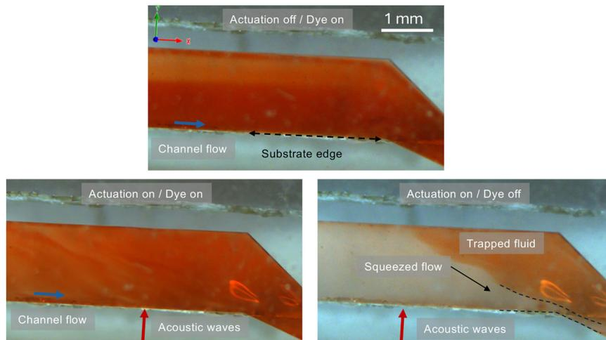
**Fig. 8** Dye mixing visualization of interaction between acoustic streaming flow and streamwise channel flow with angled channel geometry showing a large pocket of fluid trapped in closed vortices and main channel flow diverted around when dye injection is stopped (source video presented in the ESI†).
