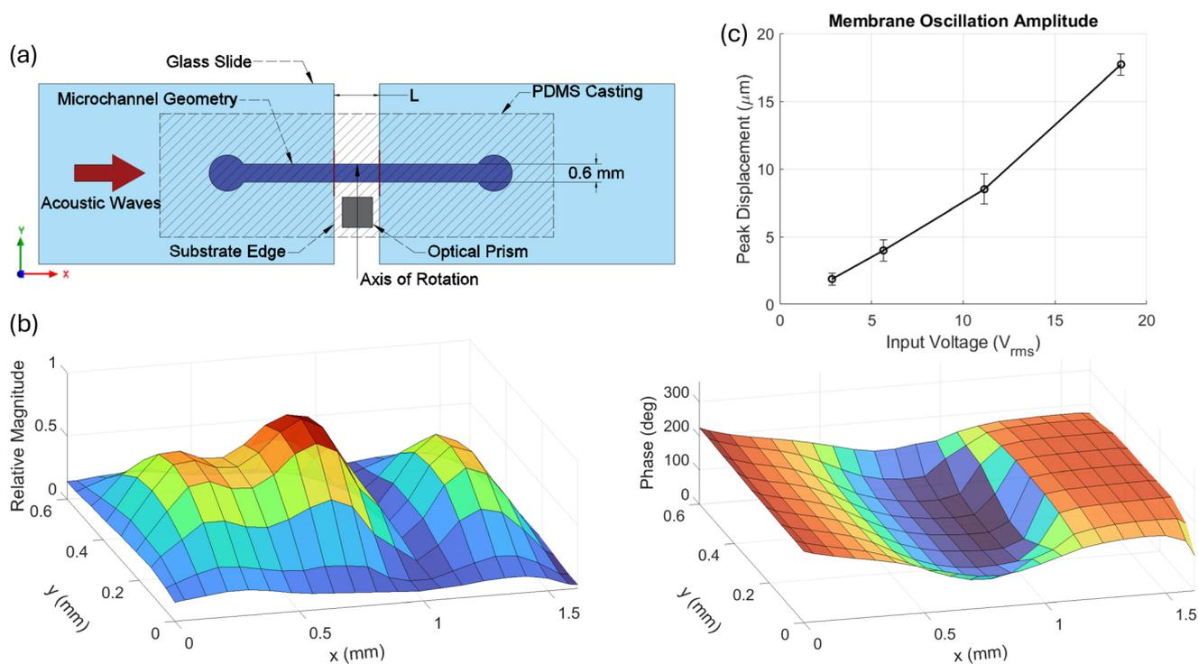
Fig. 3 (a) Top view of the testing device (the microchannel is filled with water but zero streamwise velocity,  $U = 0 \text{ m s}^{-1}$ ); (b) membrane oscillation magnitude and phase measured by LDV for  $L = 1.5$ , (c) membrane oscillation amplitude vs. input voltage.
