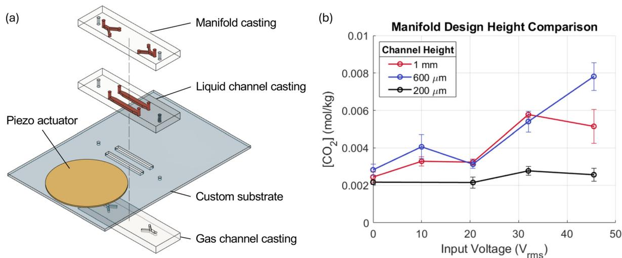
Fig. 9 (a) Schematic of the manifold dual channel gas transfer device; (b) manifold dual channel gas transfer results.
