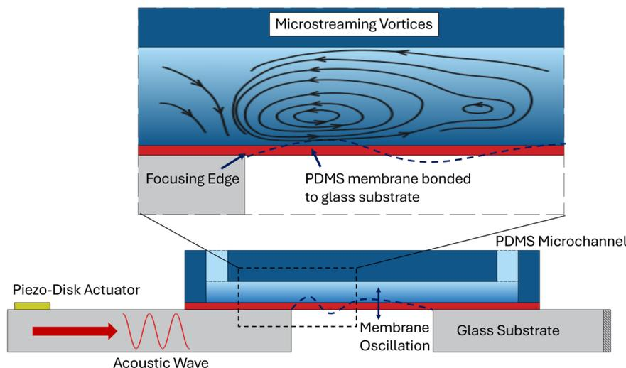
Fig. 1 Schematic diagram of the membrane microstreaming configuration.
