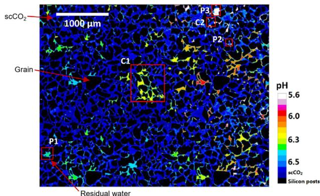
Fig. 8 Images of water pH interpreted from intensity values,  $\text{scCO}_2$ , and solid grains for 8455 pore volume of injected  $\text{scCO}_2$ . The flow direction is from left to right. Reproduced from Chang *et al.*<sup>18</sup> with permission from Elsevier, copyright 2017.
