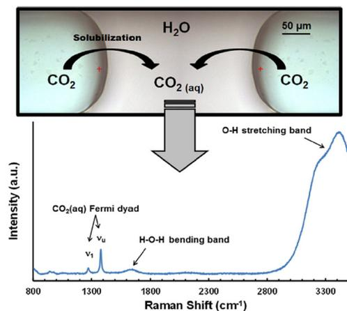
**Fig. 12** Optical image of a  $\text{CO}_2$ -water flow inside a microchannel and corresponding confocal Raman spectra within a water slug containing dissolved  $\text{CO}_2$ . Reproduced from Liu *et al.*<sup>117</sup> with permission from Elsevier, copyright 2012.
