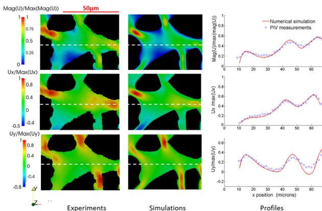
**Fig. 5** Single-phase flow in a sandstone micromodel geometry. Comparison of velocity distributions between micro-PIV measurements and numerical results. Velocity profiles plotted along the white dotted line are also compared. Here, the experimental vector resolution is  $1.76 \mu\text{m} \times 1.76 \mu\text{m}$ . Reproduced from Roman *et al.*<sup>15</sup> with permission from Elsevier, copyright 2016.
