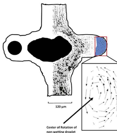
**Fig. 6** Velocity fields obtained by micro-PIV in both invading wetting and trapped non-wetting phases. Reproduced from Heshmati and Piri<sup>97</sup> with permission from Elsevier, copyright 2018.
