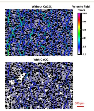
Fig. 2 Effects of crystal growth on the velocity field in the pore network. The top image shows the velocity field in the pore network without calcite crystals. The bottom image illustrates the reduced velocity field, both locally and globally, due to the deposition of calcite precipitates (white) predominantly in high-velocity zones. The velocity fields are generated with OpenFOAM.<sup>29</sup>
