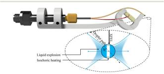
Fig. 5 Modification of 'hook' structure from Fig. 1a to produce droplets at an angle. The zoomed inset illustrates the explosion plume caused by high-pulse-energy XFELs. With sufficiently large angle  $\theta$ , these explosion debris will not intercept and accumulate on the nozzle.
