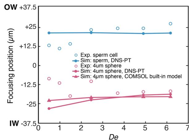
Fig. 2 Lateral focusing position of particles in a range of  $De$  numbers in the spiral channel. Experimental results for sperm cell and 4  $\mu\text{m}$  spheres are compared against the DNS-PT modelling results, and the COMSOL built-in inertial lift force model.
