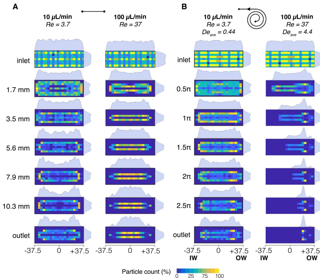
**Fig. 5** DNS-PT simulation results of the particle distribution evolution within the cross-section of the  $75 \mu\text{m} \times 25 \mu\text{m}$  straight and spiral channels presented as heatmaps for (A) straight channel at  $Q = 10$  and  $100 \mu\text{L min}^{-1}$  ( $Re = 10$ , and  $Re = 100$ , respectively) and (B) spiral channel at  $Q = 10$  and  $100 \mu\text{L min}^{-1}$  ( $Re = 10$ ,  $De_{\text{ave}} = 0.44$  and  $Re = 100$ ,  $De_{\text{ave}} = 4.4$ , respectively).
