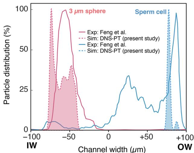
Fig. 4 Lateral particle distribution at the channel outlet for sperm cells and  $3 \mu\text{m}$  spheres in a  $200 \mu\text{m} \times 50 \mu\text{m}$  spiral channel. Experimental observations by Feng *et al.* (solid line) vs. DNS-PT modelling results (dashed line). Note that Feng *et al.* conducted experiments using human sperm cells, while the DNS-PT model is based on bovine sperm cell dimensions.
