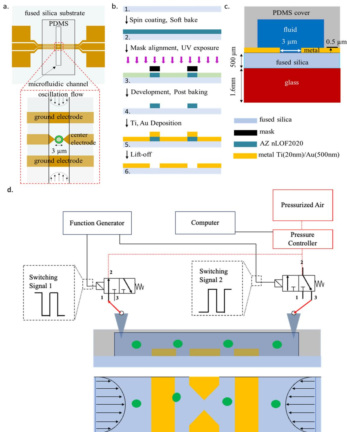
Fig. 2 (a) Schematic top view of CPW (b) microfluidic device integrated with CPW fabrication process (c) description of sealing the microfluidic channel on the substrate. (d) Schematic of the oscillatory system.
