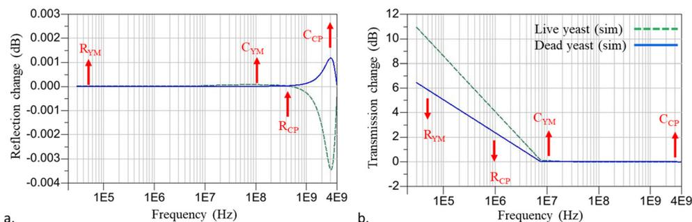
**Fig. 7** Equivalent circuit parameters sensitivity with respect to the frequency in *S*-parameter spectrum for (a) reflection and (b) transmission changes up to 4 GHz. The circuit elements comprise yeast membrane resistance ( $R_{YM}$ ), yeast membrane capacitance ( $C_{YM}$ ), cytoplasm resistance ( $R_{CP}$ ), and cytoplasm capacitance ( $C_{CP}$ ). The direction of the arrows indicates each parameter's incremental effect at the frequency where the effect is most significant.
