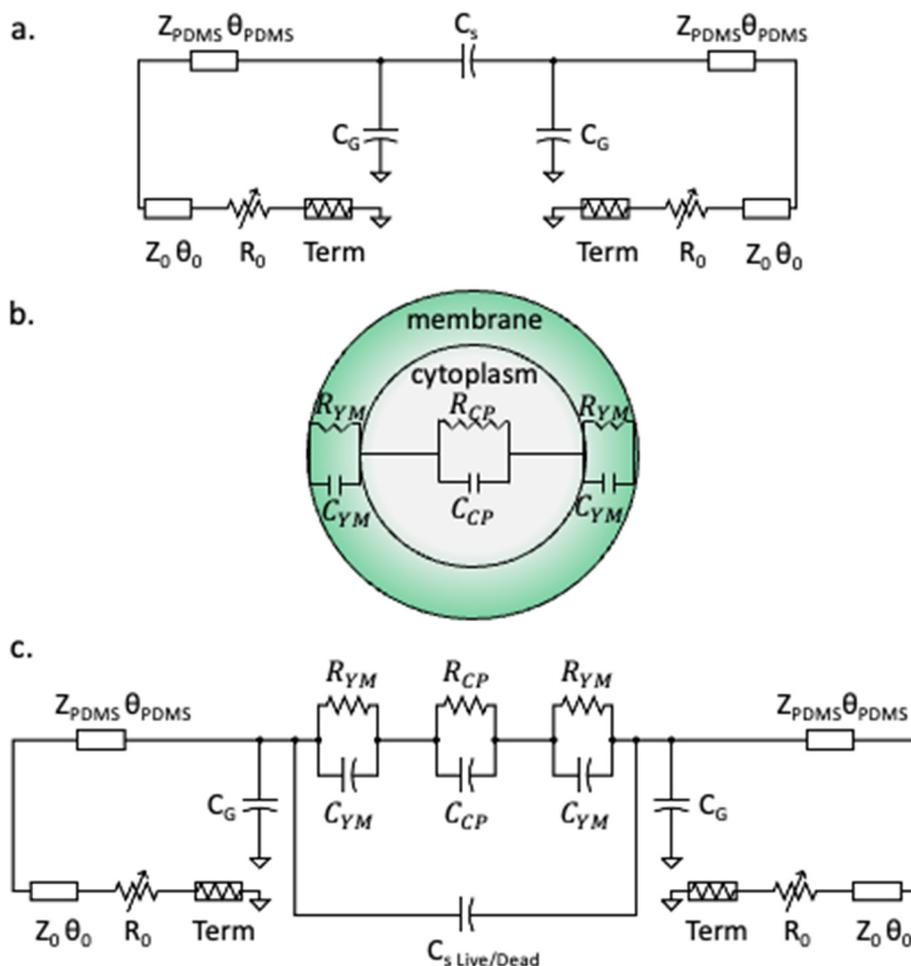
**Fig. 3** (a) Equivalent circuit of the coplanar waveguide (CPW) comprising distributed sections under PDMS and air (b) equivalent circuit of the yeast with 4 equivalent circuit elements comprising yeast membrane resistance ( $R_{YM}$ ), yeast membrane capacitance ( $C_{YM}$ ), cytoplasm resistance ( $R_{CP}$ ), and cytoplasm capacitance ( $C_{CP}$ ). (c) Equivalent circuit of the coplanar waveguide with a yeast-trapped between the CPW signal electrode gaps.
