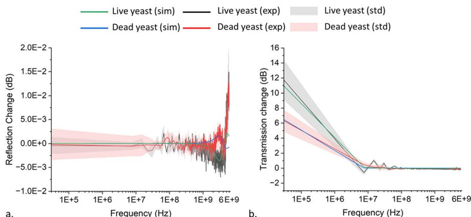
Fig. 6 (a) Reflection and (b) transmission magnitude changes for live and dead single yeast trapped between coplanar waveguide (CPW).
