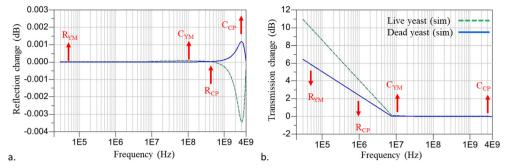
Fig. 7 Equivalent circuit parameters sensitivity with respect to the frequency in S-parameter spectrum for (a) reflection and (b) transmission changes up to 4 GHz. The circuit elements comprise yeast membrane resistance  $(R_{YM})$ , yeast membrane capacitance  $(C_{YM})$ , cytoplasm resistance  $(R_{CP})$ , and cytoplasm capacitance  $(C_{CP})$ . The direction of the arrows indicates each parameter's incremental effect at the frequency where the effect is most significant.
