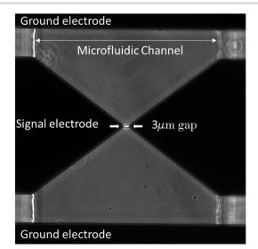
Fig. 5 Micrograph of trapped yeast by dielectrophoresis (DEP) between the coplanar wave guide (CPW) electrode.
