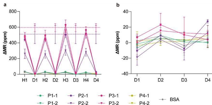
**Fig. 6** (a) Regeneration of chips for repeated measurements of target groups P2 and P3 using 40% DMSO. H and D indicate the signals obtained after hybridization and denaturation in each cycle, respectively. The dashed lines represent the average hybridization signals (purple: P2 and red: P3) obtained before regeneration. (b) Remaining signals after each denaturation cycle using 40% DMSO. The error bars represent the SD of four identical sensors ( $n = 4$ ).
