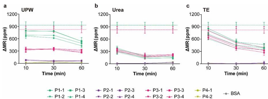
**Fig. 3** Hybridization signals from the chips regenerated using (a) UPW, (b) urea solution, and (c) TE buffer at 90 °C for different denaturation times (10, 30, and 60 min). After regeneration, the chips were incubated with target groups P1 and P3. The dashed lines indicate the average hybridization signals from new chips without any regeneration (green: P1 and red: P3). The error bars represent the SD of four identical sensors ( $n = 4$ ).
