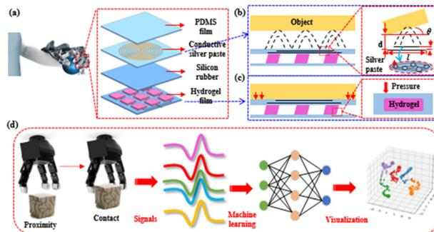
Fig. 1 (a) Schematic diagram of FDMSs for robot grasping manipulation. (b) Working principle of proximity perception of the flexible dual modal sensor. (c) Working principle of contact pressure perception of flexible dual modal sensors. (d) Robot electronic skin based on flexible dual modal sensors achieves multifunctional perception through machine learning.
