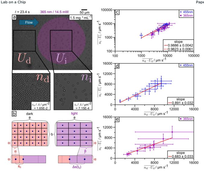
Fig. 5 a) Snapshot of optical micrograph from Video S3.† b) Schematic representation of free space per particle without (left) and with (right) illumination. c) Log-log plot of the left side of egn (1) against the right side for blue and UV illumination with respective linear regressions d and e) linear plot of the left side of eqn (1) against the right side for blue (455 nm) and UV (365 nm) light with respective linear regressions.
