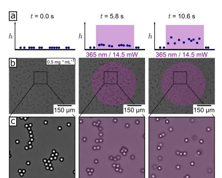
Fig. 2 (a) Cartoon of the side view of initially sedimented microparticles upon light illumination, interpreted from the (b and c) snapshot series of optical micrographs from Video  $S1^{+}$  at the time t = 0.0, 5.8 and 10.6 s. No fluid flow is applied. The purple area illustrates the illuminated area.
