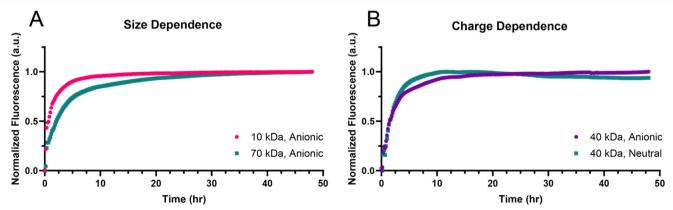
Fig. 7 Optical sensing allows real-time multiplexing of fluorescently tagged analyte. A) Size-dependent diffusion rate of fluorescently tagged dextran sensed simultaneously. A 10 kDa dextran (tagged with Alexa Fluor 647) diffused more rapidly through the semi-permeable membrane compared to the 70 kDa dextran (tagged with fluorescein). B) Charge-dependent diffusion rate of dextran of similar size (neutral: Texas Red; anionic: fluorescein).
