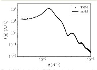
Fig. 4 SAXS signal of the TM50 dispersion before compression (symbols) and corresponding model (line) for a reservoir salt concentration  $c_{\rm res}$  = 5 mM. The optimized model parameters are: average radius a = 14.2 nm, polydispersity 1.46 nm, volume fraction  $\phi$ = 0.082, pH = 9.02 (corresponding to a bare surface charge density  $\sigma$
