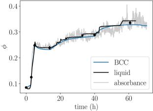
Fig. 6 Volume fraction  $\phi$  as a function of time during compression in the microfluidic chip. The different line colors correspond to different approaches to estimate the volume fraction, as described in the text. The black circles correspond to the 2D SAXS patterns reported in Fig. 3. Their  $\phi$  value is the average of the "liquid" and "BCC" values.
