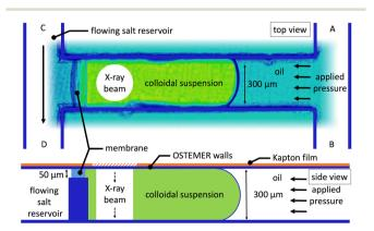
Fig. 1 Central part of the microfluidic setup with a drop of colloidal suspension trapped on the membrane. The size of the X-ray beam (250  $\mu$ m) is represented approximately. The hatched portion of the Kapton film was present in the main experiment reported here, but could be removed in the preliminary experiment reported as ESI.†
