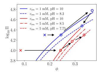
Fig. 7 Equation of state of TM50 colloids measured in the present microfluidic chip (open symbols), and calculated theoretically (lines, see main text for the details). For calculations, a=14.2 nm. The two crosses show the initial volume fraction of the suspension and do not correspond to equilibrium data. The black arrows show the path followed by the dispersion in the microfluidic chip.
