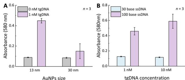
**Fig. 4** Signal and noise (background absorbance) obtained with probe sticks in dual-enzymatic reactions depending on (A) size of AuNPs used for probe stick modification with 100 base ssDNA, and (B) length of ssDNA used for conjugation of ALP to 13 nm AuNPs.
