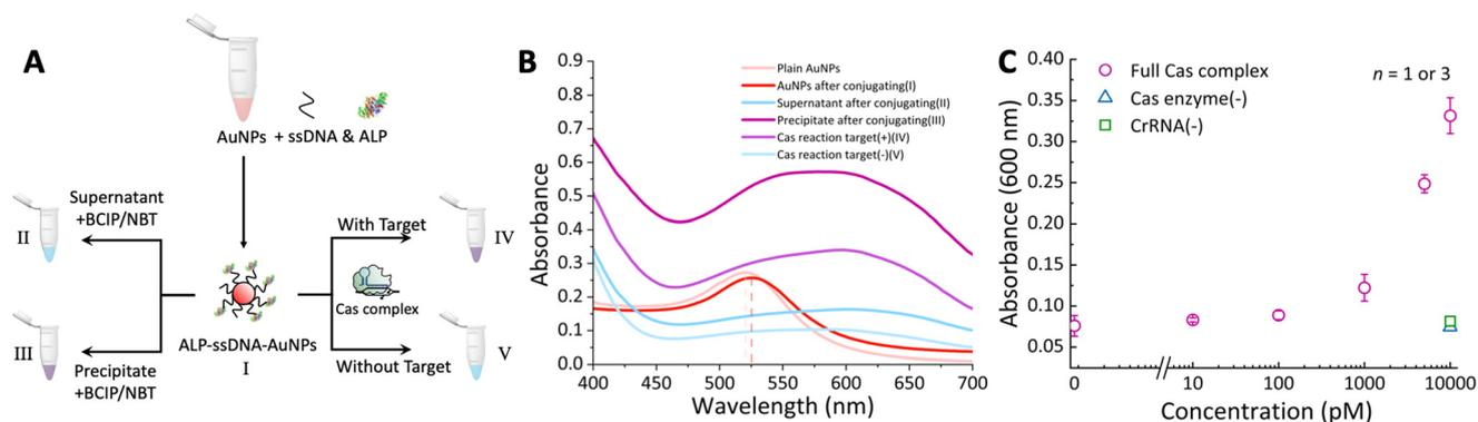
**Fig. 3** (A) Workflow of evaluating AuNPs–ssDNA–ALP conjugation and target DNA responsiveness; (B) absorption spectra for each solution described in (A); (C) target DNA concentration-dependent response curve after 30 min of Cas cleavage reaction and 20 min of ALP enzymatic reaction in aqueous solutions.
