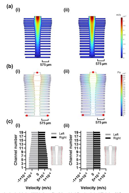
Fig. 2 Redesign of the spine-inspired design. (a) Velocity profile of the original (i) and optimized (ii) design. (b) Pressure profile of the original (i) and optimized (ii) design. (c) Velocity vector in each reaction site (red circles) for the original (i) and optimized (ii) design. Simulations are run using fully developed laminar flow at 100  $\mu$ L min<sup>-1</sup> flow rate.
