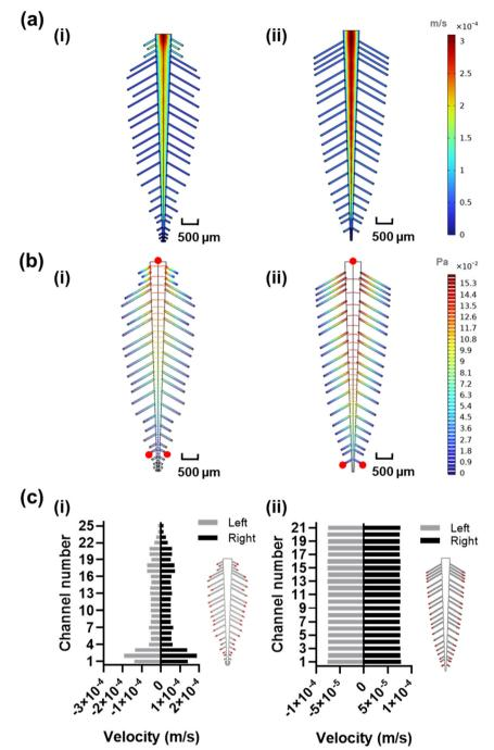
Fig. 3 Redesign of the leaf-inspired design. a) Velocity profile of the original (i) and optimized (ii) design. b) Pressure profile of the original (i) and optimized (ii) design. c) Velocity vector in each reaction site (red circles) for the original (i) and optimized (ii) design. Simulations are run using fully developed laminar flow at 100 µL min<sup>-1</sup>
