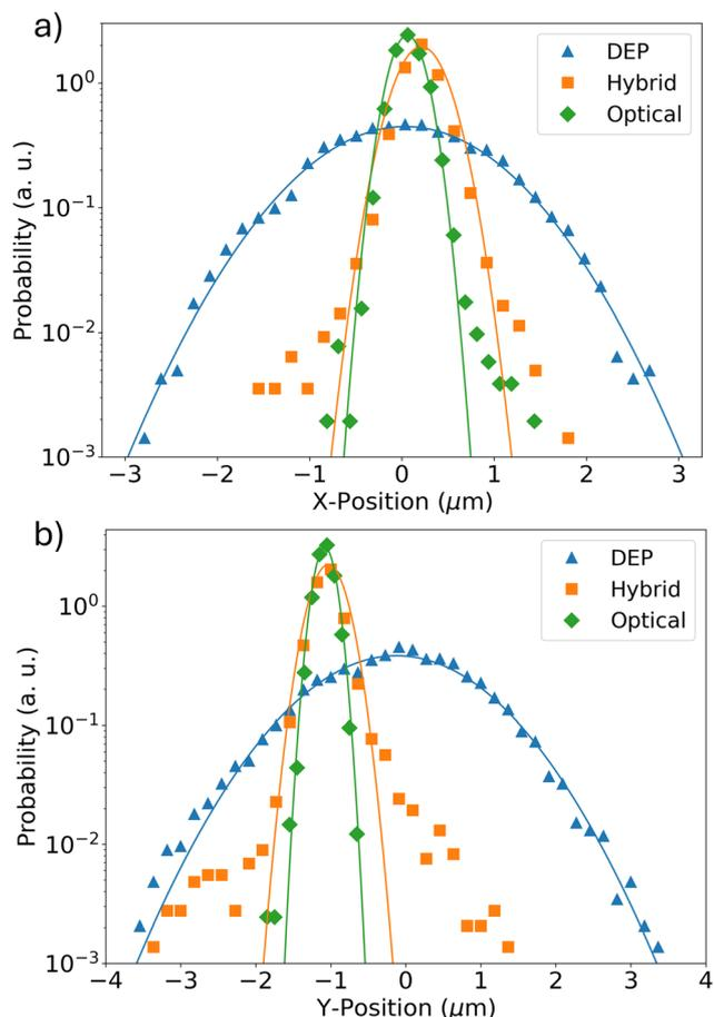
**Fig. 3** Hybrid DEP–optical trap. 1D histograms of the (a)  $x$  and (b)  $y$  positions of a  $1\ \mu\text{m}$  polystyrene particle. The blue triangles correspond to the DEP trap, the green diamonds to the optical trap, and the orange squares to the combined trap. The solid lines represent fits to Gaussian functions. The power of the laser beam was the same ( $1\ \text{mW}$ ) in both the experiments performed with the optical and hybrid traps.
