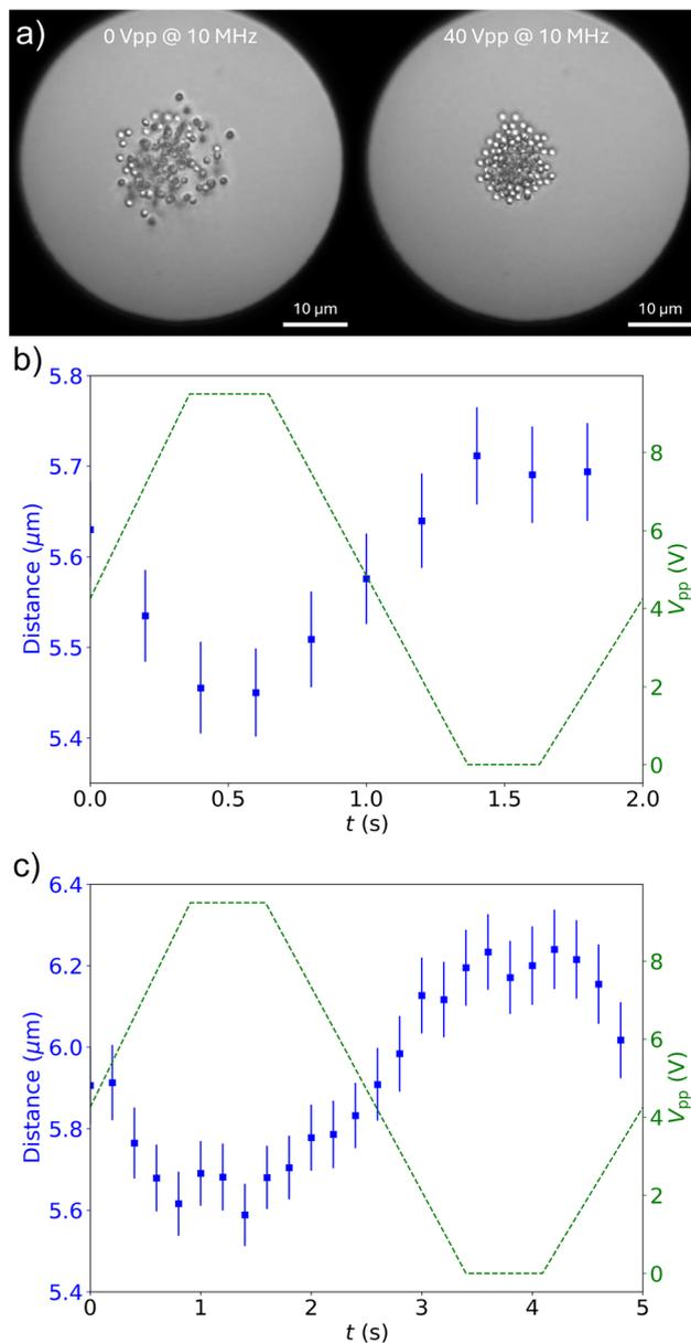
Fig. 8 Trap modulation. (a) Cycles of expansion (left) and compression (right) of  $1 \mu\text{m}$  polystyrene particles. Average distance between the  $1 \mu\text{m}$  polystyrene particles for 2 (b) and 5 s (c) period cycles, respectively. The green dashed line is the modulated amplitude of the feed voltage, while the blue dots are the averaged distance between every two particles, vs. cycle time. The error bars represent the standard deviation from the repeated cycles.
