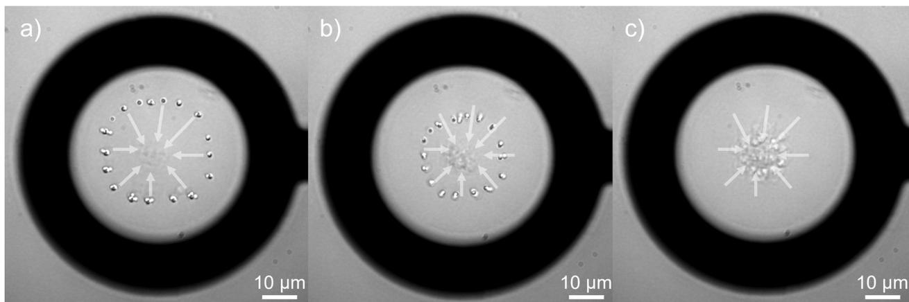
**Fig. 4** Controlled loading of the DEP trap from optical tweezers. (a)  $1\ \mu\text{m}$   $\text{SiO}_2$  particles optically trapped within the DEP trap. (b and c) After we switched off the optical traps, the particles quickly moved to the centre of the DEP trap. The white arrows indicate the net particle displacement throughout the video.
