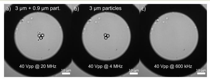
Fig. 5 Selective trapping. (a) The experiment starts with four 0.9 μm ProMag® 1 particles and three 3.1 μm ProMag® 3 particles trapped with an electric field of 40 Vpp and 20 MHz. (b) At a given time, we changed the frequency to 4 MHz, kicking out the small particles. (c) Larger particles can also be expelled from the trap by reducing the frequency down to 600 kHz.
