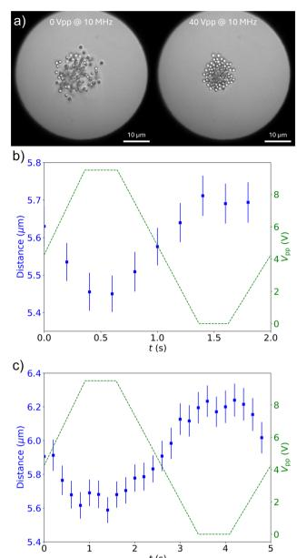
Fig. 8 Trap modulation. (a) Cycles of expansion (left) and compression (right) of 1  $\mu$ m polystyrene particles. Average distance between the 1 μm polystyrene particles for 2 (b) and 5 s (c) period cycles, respectively. The green dashed line is the modulated amplitude of the feed voltage, while the blue dots are the averaged distance between every two particles, vs. cycle time. The error bars represent the standard deviation from the repeated cycles.
