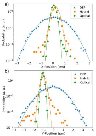
Fig. 3 Hybrid DEP-optical trap. 1D histograms of the (a) x and (b) y positions of a 1  $\mu$ m polystyrene particle. The blue triangles correspond to the DEP trap, the green diamonds to the optical trap, and the orange squares to the combined trap. The solid lines represent fits to Gaussian functions. The power of the laser beam was the same (1 mW) in both the experiments performed with the optical and hybrid traps.
