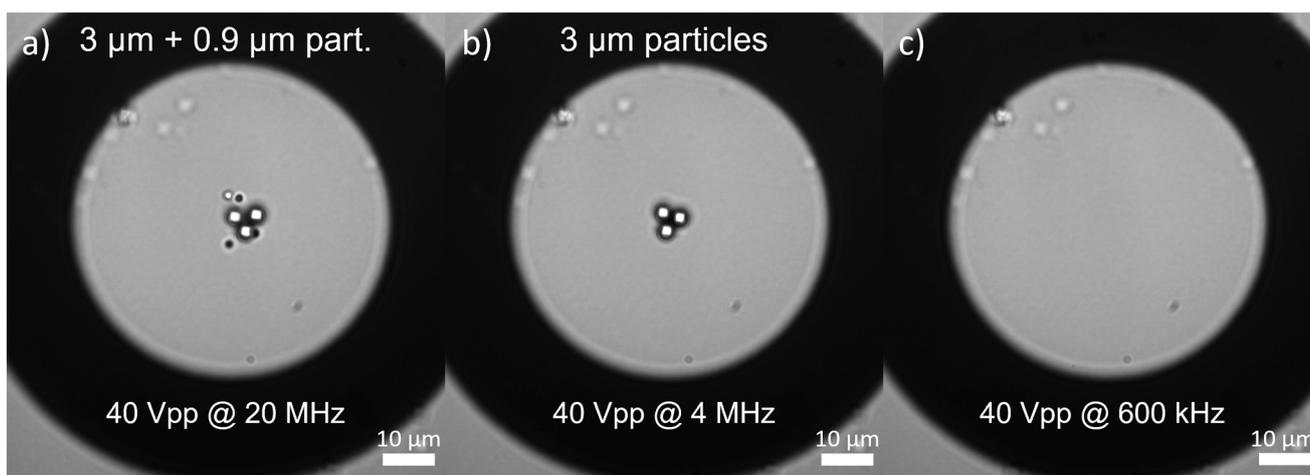
**Fig. 5** Selective trapping. (a) The experiment starts with four  $0.9\ \mu\text{m}$  ProMag® 1 particles and three  $3.1\ \mu\text{m}$  ProMag® 3 particles trapped with an electric field of  $40\ \text{V}_{\text{pp}}$  and 20 MHz. (b) At a given time, we changed the frequency to 4 MHz, kicking out the small particles. (c) Larger particles can also be expelled from the trap by reducing the frequency down to 600 kHz.
