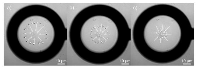
Fig. 4 Controlled loading of the DEP trap from optical tweezers. (a) 1 μm SiO<sub>2</sub> particles optically trapped within the DEP trap. (b and c) After we switched off the optical traps, the particles quickly moved to the centre of the DEP trap. The white arrows indicate the net particle displacement throughout the video.
