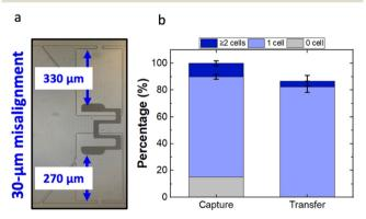
**Fig. 6** (a) Brightfield micrograph of a purposely misaligned PDMS-electrode assembly with pocket-electrode gap measured with corresponding microscope settings. (b) Bar graph showing percentage of empty, singly, and multiply occupied pockets and singly and multiply occupied chambers out of occupied pockets. Cell concentration of  $8\times10^5$  cells per mL, 90 nL min<sup>-1</sup> flow rate, applied voltage of  $66.2\,\mathrm{V_{p-p}}$  at  $100\,\mathrm{kHz}$ .
