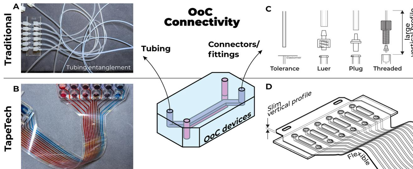
**Fig. 1** Comparison of OoC connectivity between traditional tubing connectors and TapeTech connectors. A) Photograph showing tubing entanglement in a traditional microfluidic setup. B) Photograph of TapeTech ribbon, showcasing the organized, clutter-free setup. C) Schematic illustration of conventional commercially available connectors with their large vertical profiles. D) Schematic illustration of the TapeTech assembly, highlighting its slim vertical profile and streamlined design.
