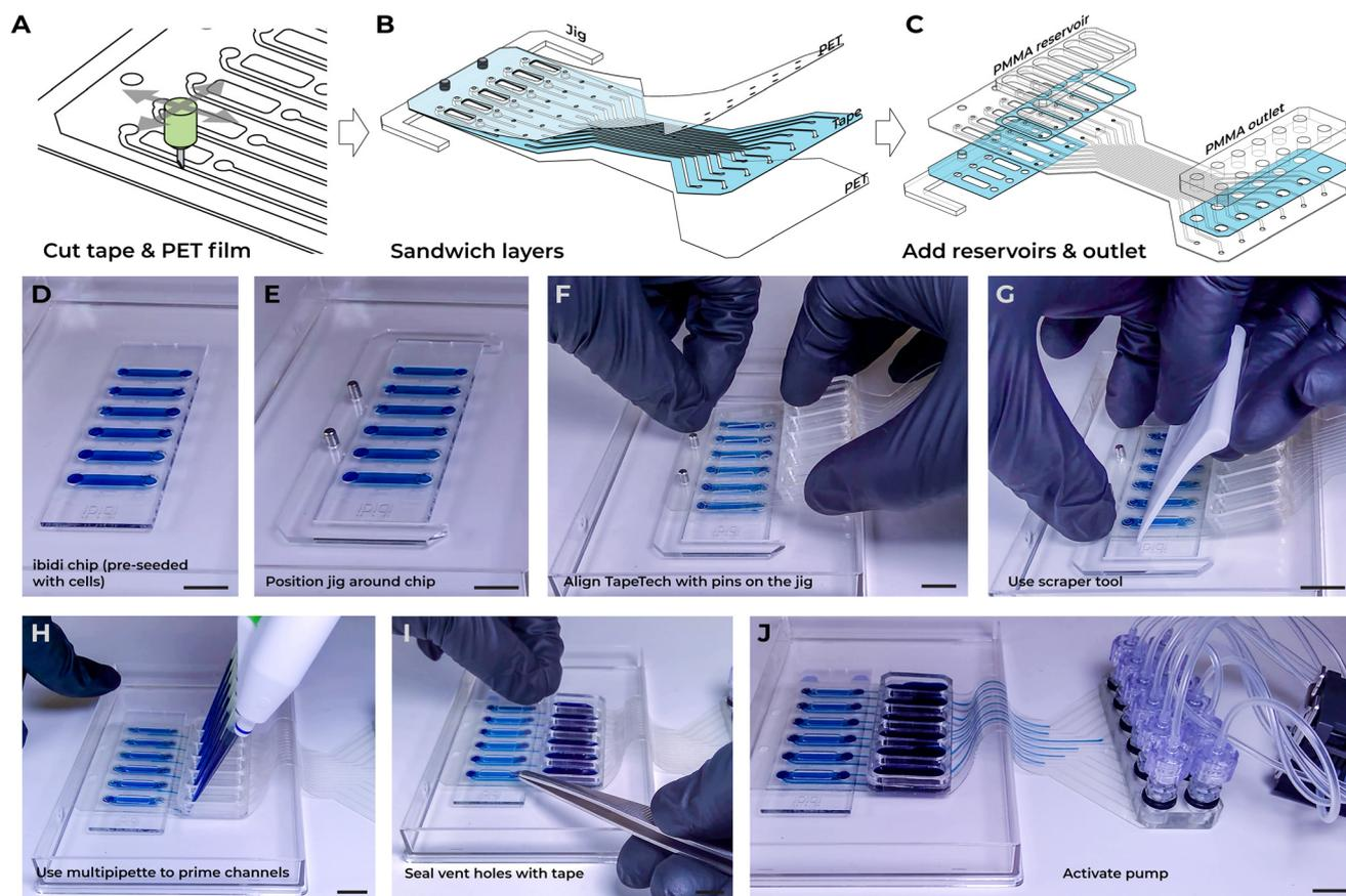
**Fig. 5** Fabrication and assembly process of TapeTech connectors. A) Schematic illustration of the cutting process for double-sided tape and PET films. B) Alignment and layering of multiple tape and PET film layers using a jig for precise assembly. C) Integration of additional components, such as reservoirs and outlets, with double-sided tape. D–J) Sequential snapshots representing the key steps involved in connecting the TapeTech assembly to the ibidi 6-channel chip. Scale bar: D–J) 10 mm.
